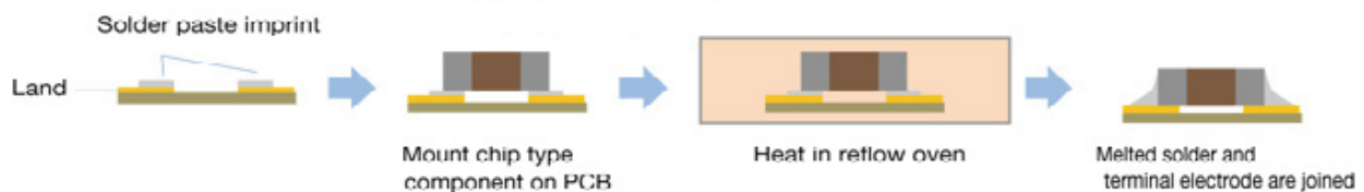
Figure 11 Reflow soldering process
