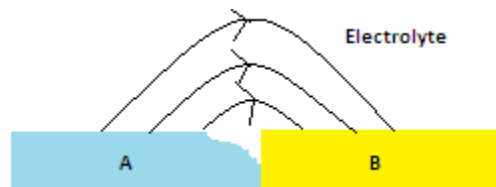
Figure 15 Galvanic corrosion: metal A, less noble, acts as the anode; metal B, more noble, acts as a cathode
