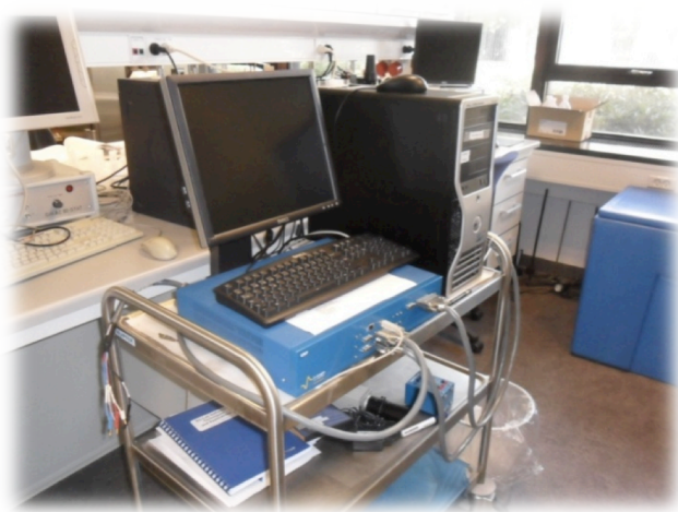
Figure 27 BioLogic VSP multichannel potentiostat
