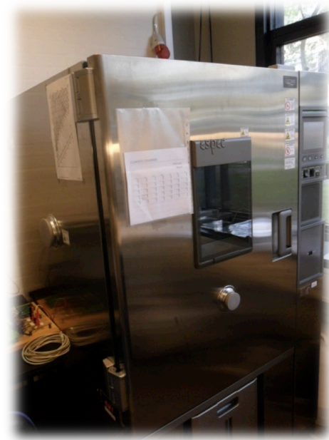
Figure 23 ESPC PL-3KPH climatic chamber
