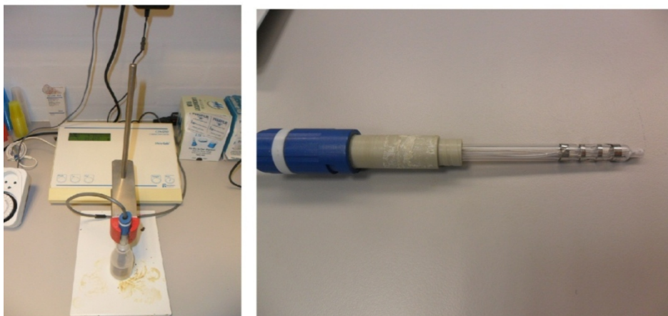
Figure 28 CDM210 conductivity meter (on the left); 4-electrode conductivity cell
