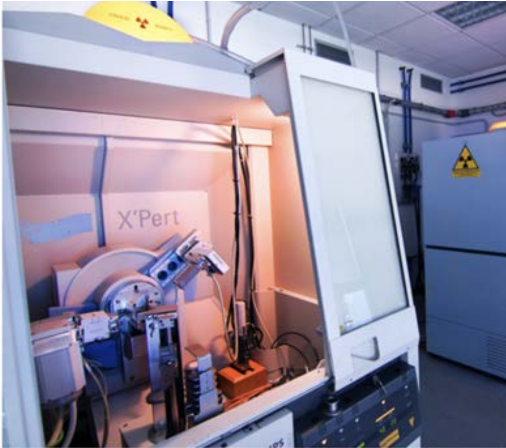
Fig. 7 – Philips X'Pert PRO diffractometer, Bragg-Brentano geometry with Bragg-Brentano HD optics, cobalt source, X'Celerator detector, and Anton Paar HTK16 hot stage. (source: https://www.geoscienze.unipd.it/diffrattometria-x-polveri )
