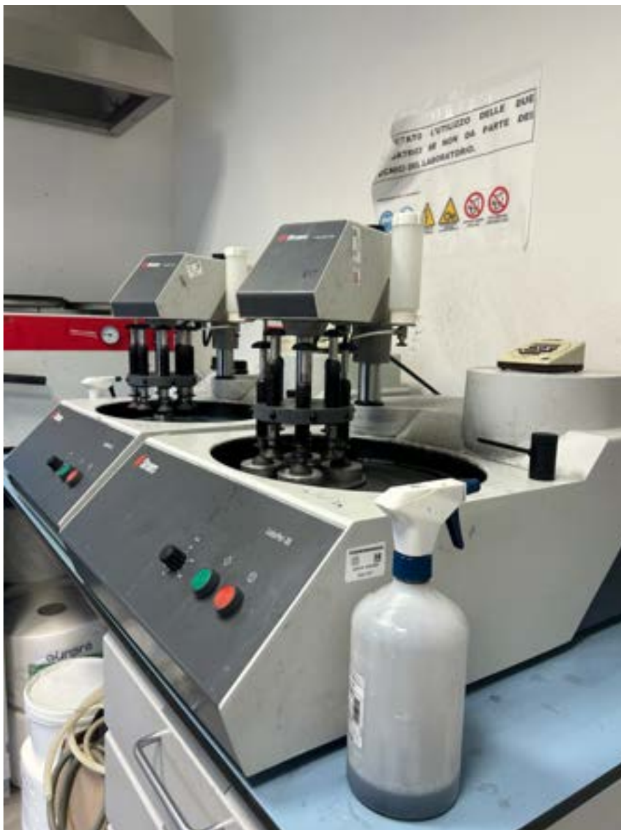
Fig. 10 – Struers LaboPol-35 polishing machine (photo by Sokolova E.)
