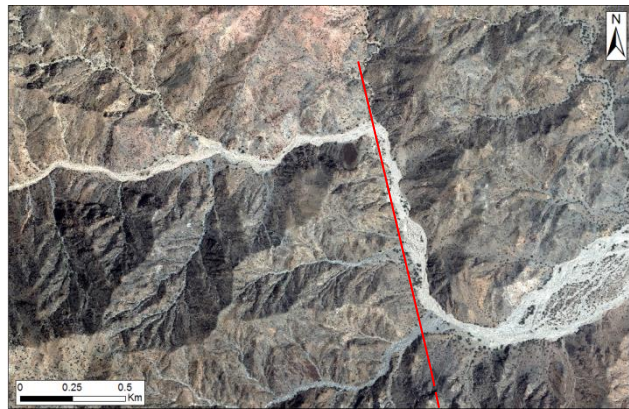
Figure 64. An example of a structural lineament deduced from the surface drainage analysis.
