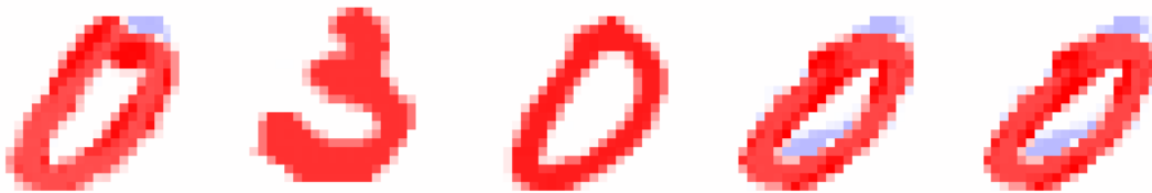
Figure 6.12: Feature maps of the five most active hidden neurons given the input digit shown in Fig. 6.10. These five neurons are those with an activation greater than 95% the maximum value.
