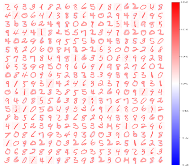
Figure 6.3: Feature maps learned during the bio-training. These feature maps, as anticipated before, can be understood by humans because are digit prototypes. Red pixels means positive weights, while blue pixels means negative ones.
