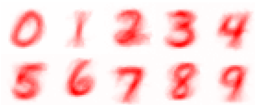
Figure 6.17: Feature maps of the second layer obtained from an ANN trained with the proposed algorithm. Each output neuron "sees" its corresponding digit through the weights of the network.
