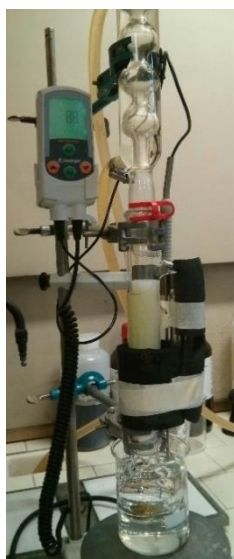
Figure 3.42 Soxhlet apparatus used for the polyhydroxyalkanoates extraction
