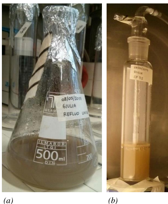
Figure 3.7 (a) Sterilized real medium (b) Final day of batch experiment of Chlorella in sterilized medium
