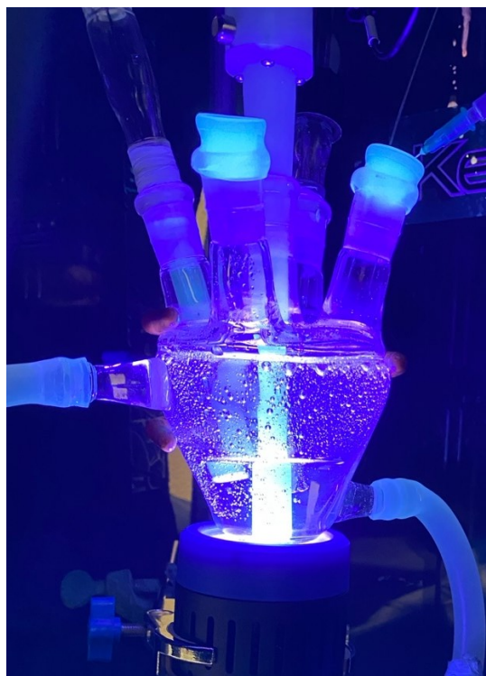
Figure 7. Digital picture of the setup for CV electrophotochemistry experiments.
