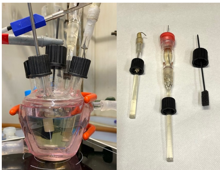
Figure 8. Left: Electrochemical setup for the synthesis of radical cation salts. Right: RE, CE, and WE electrodes used in the synthesis.
