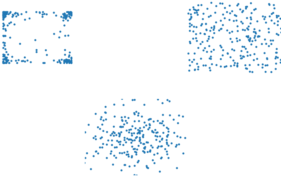
Figure 5.4: Other examples of plots for n=256 case: the first one represents the transmitting channel case, the second one an uniform jammed channel and the third one a Gaussian jammed channel.
