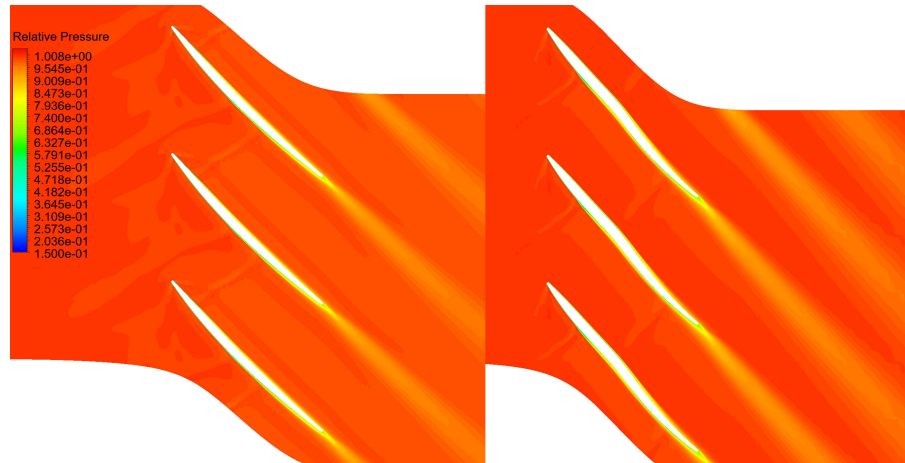
Figure 3.65: Relative total pressure ratio contour for the individuals from the first optimization (left) and second (right) under design conditions (first design point).
