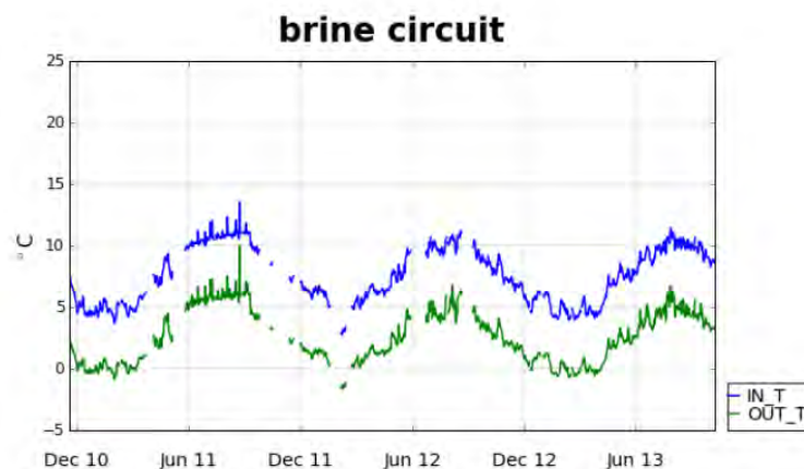
Figure 14 Measurements of brine-water temperature (Marek Miara, 2011)
