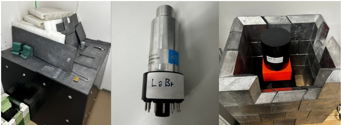
Figure 2 – Experimental equipment used in the activation measurements: (a) shielded irradiation setup housing the Am–Be neutron source, (b) LaBr 3 (Ce) detector, and (c) NaI(Tl) detector.
