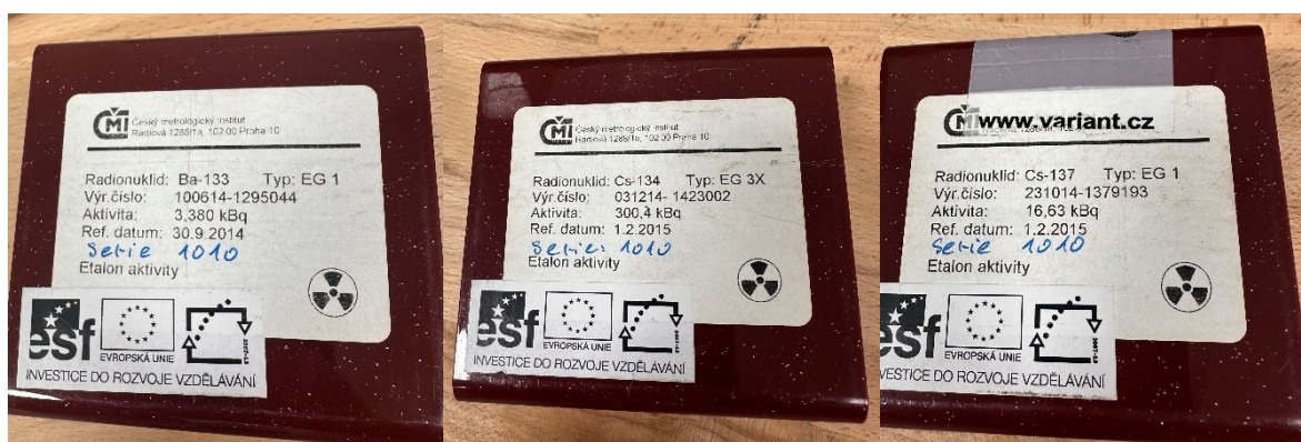
Figure 5 – Calibration sources used for efficiency determination ( 133 Ba, 134 Cs, 137 Cs)
