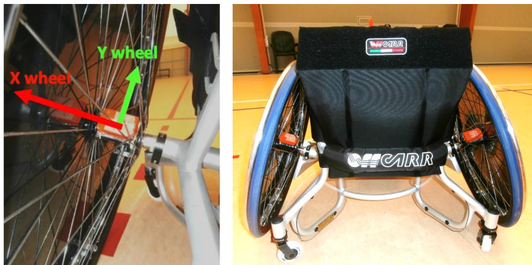
Figure 41. Sensors in the wheels. Left: wheel system of reference; right: sensors fixation.
