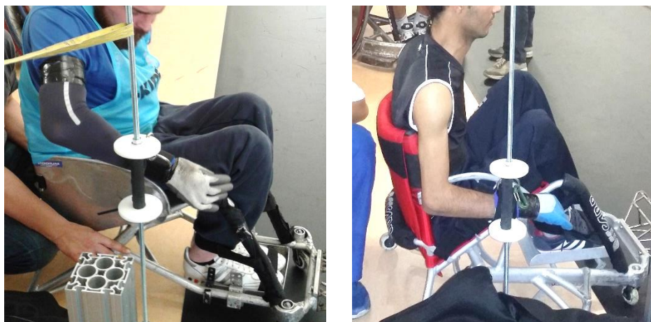
Figure 30. Elbow extension test. Left: wrong way of execution (shoulder abduction, less than 90° of elbow flexion, the applied force is not parallel to the beam). Right: right way of execution (no trunk rotation, 90° of elbow flexion, force parallel to the beam).
