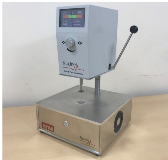
Figure 4.1 ATAC NuLine cone and Plate viscometer used to measure the viscosity of the PAA solution.
