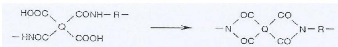
Figure 5.3 Imidation by PAA cyclization to form Polyimide (PI).
