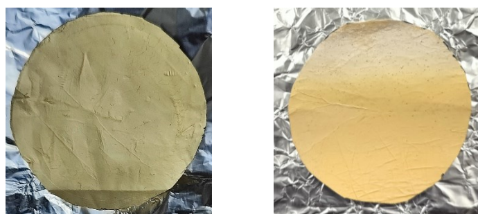
Figure 6.9 Homogeneous and uneven TiO 2 dispersion in a PI membrane.
