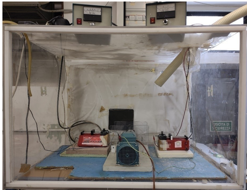
Figure 4.3 Electrospinning setup used for the production of all the membranes.
