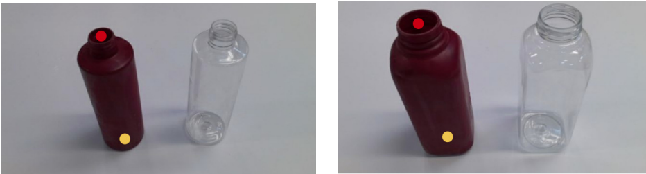
Figure 4.2. bottle_1 and bottle_2 objects, with the keypoints used by Keypose, next to an opaque counterpart
