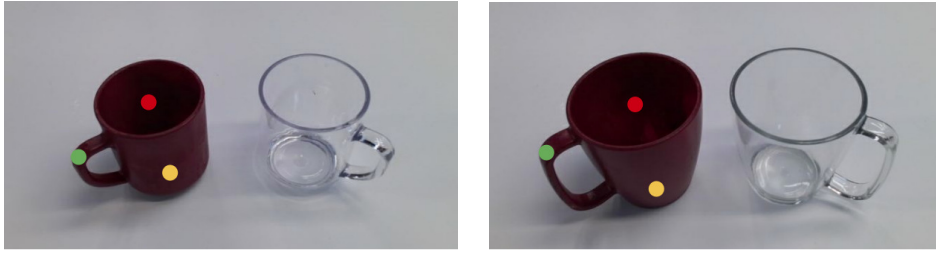
Figure 4.5. mug_2 and mug_3 objects, with the keypoints used by Keypose, next to an opaque counterpart
