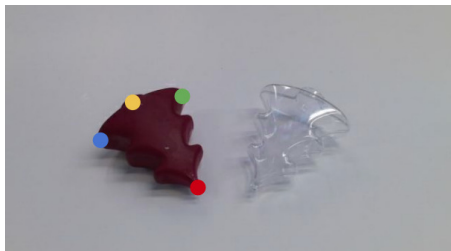
Figure 4.8. tree_0 object, with the keypoints used by Keypose, next to an opaque counterpart
