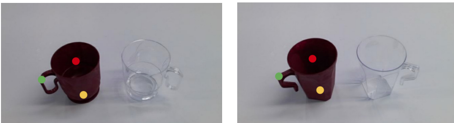
Figure 4.4. mug_0 and mug_1 objects, with the keypoints used by Keypose, next to an opaque counterpart
