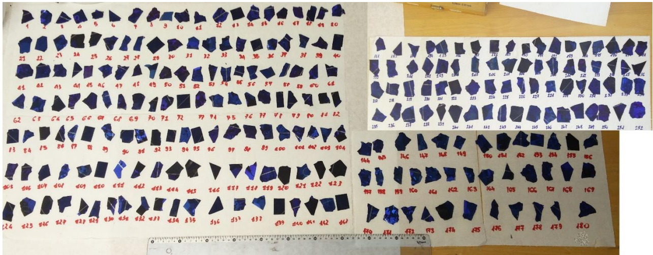
Fig. 4.2 All the 252 samples for the back-side etching treatment (a 50 cm long ruler for scale)
