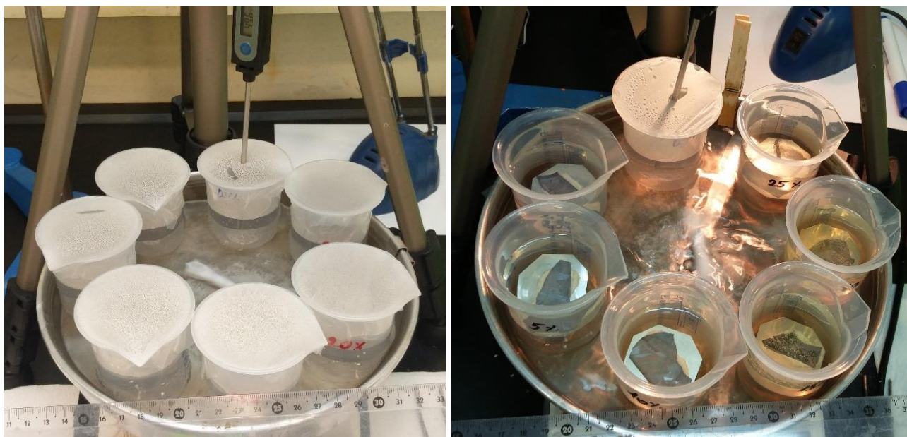
Fig. 4.4 (left) Heating of the different solutions (in this case at 50°C); (right) Etching treatment on the samples (in this case at 40°C for 1 hour)
