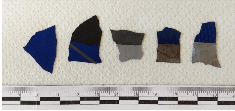
Fig. 4.5 (from left to right) As-received sample; half of the surface is covered with a high-temperature resistant paint; sample treated in 10% HF solution for 15 minutes; paint removed with nitro thinner; treated sample in sodium hydroxide solution.
