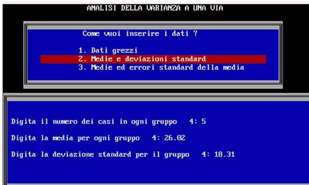
Figure 15: Primer program screenshot. Providing essential data for ANOVA analysis, including the number of groups, number of the examined cases in each group, their means, and standard deviation.
