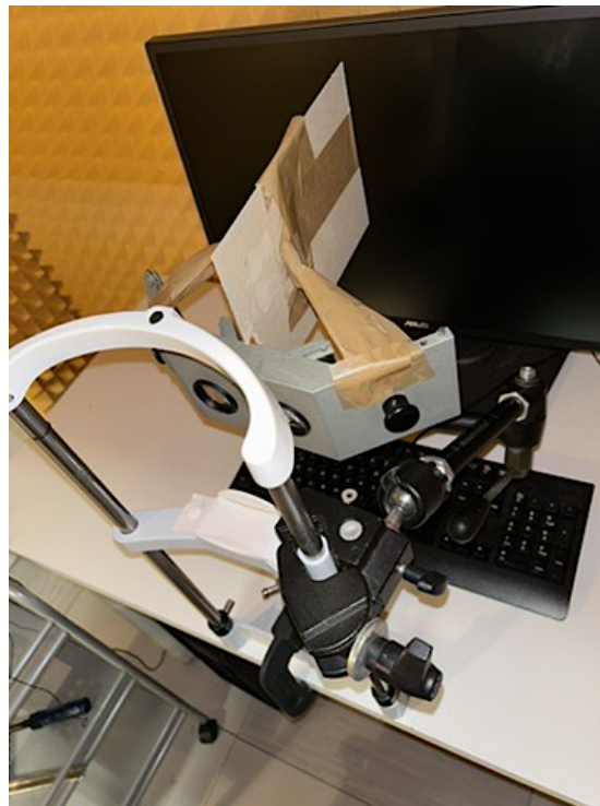
Figure 8. This image shows a side view of the stereoscopic mirror to see how the piece of cardboard was attached to the rest of the equipment.
