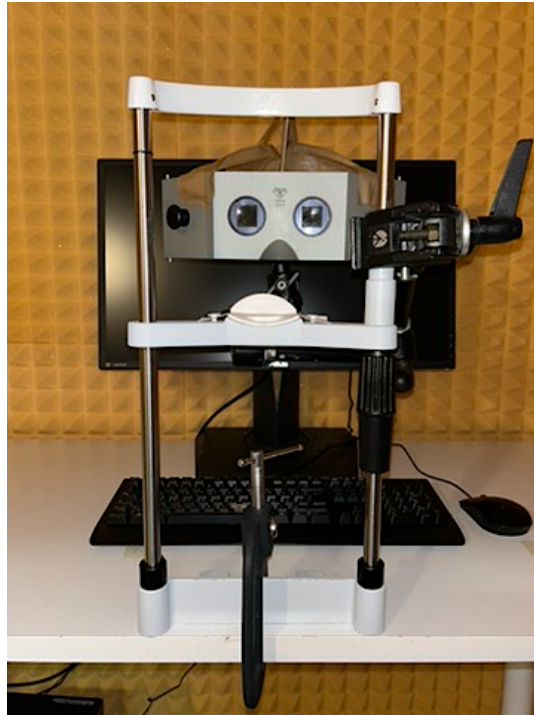
Figure 7. Frontal view of the experimental setting. The chin guard helps to support the participant's head for the duration of the procedure. It is also possible to see the stereoscopic mirror attached to the chinrest.
