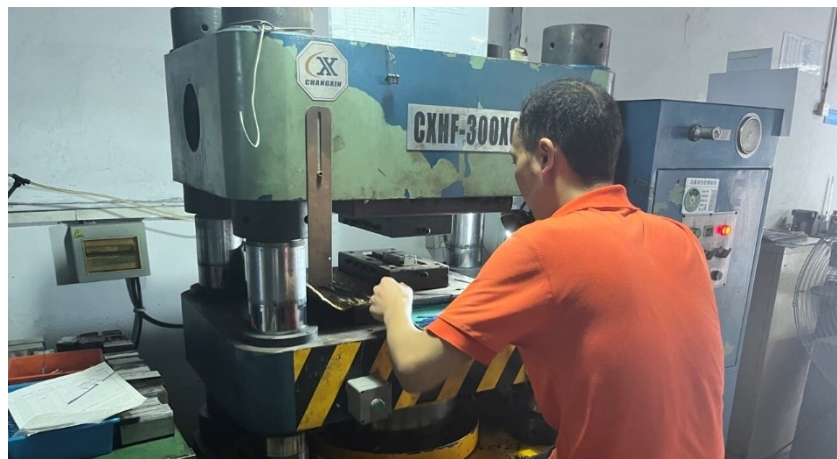
Figure 17 Stamping machine for eyeglasses components shaping. 13
