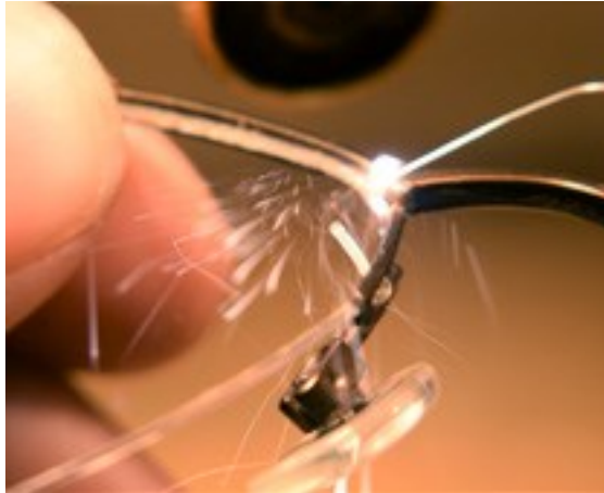
Figure 18 Laser soldering of eyeglasses components. 14
