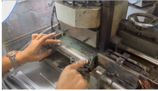
Figure 21 Metal core insertion in CA temples. 17
