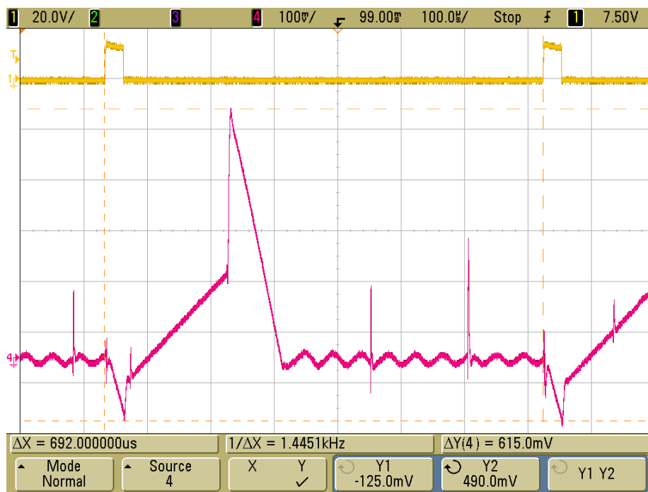
Figure 4.6: Measurement of the static behaviour of the converter, showing a complete switching cycle. The displayed waveforms are the LS-SW gate signal (yellow) and the output current (magenta). The current probe is set to 100mV/A. The cursors measure the positive and the negative peak output current, which result i_p = 4.9\text{A} and i_r = 1.25\text{A} respectively.
