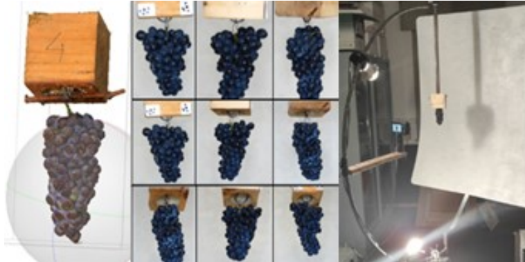
Figure 3.1. Image acquisition device, photos sequence, and final 3D virtual model.
