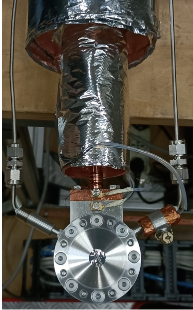
(a) Cryogenic target utilized in the experiment. The image presents the aluminum body, the copper finger and the pipes that supply the helium gas.
