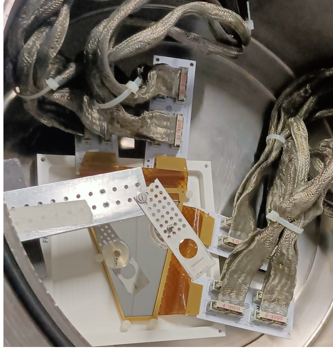
Figure 2.4: Setup inside the vacuum chamber. The GRIT detector, adapters, and the triple alpha source (on the top) are depicted in the image. For a better visualization of all the elements, notice that there is a reflection on the trapezoidal detector (see Figure 1.7a).
