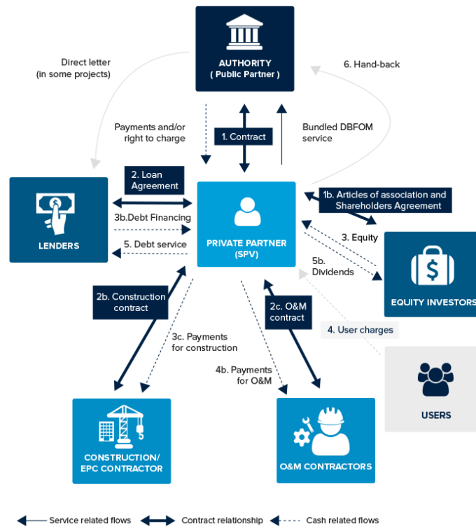
Figure 8: Public – Private Partnership contracts creation and payments timetable Source: PPP Certification Website
