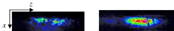
Figure 4.8: Images of group D, wrote in titanium waveguide. a) D1 guide, created in a crystal defect. b) D2 guide, where the propagation is mono-mode, and where a defect owed to the crystal is present.
