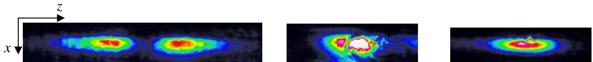
Figure 4.7: Images of group C, wrote in titanium waveguide. a) C1 guide, characterized by a multi-mode propagation of light. b) C2 guide, where the propagation is mono-mode, but a defect owed to the crystal is presented. c) C3 guide, with a mono-mode propagation.
