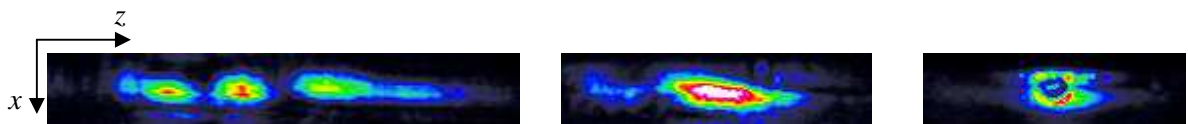
Figure 4.6: Images of group A, written in titanium waveguide. a) A1 guide, characterized by a multi-mode propagation of light. b) A2 guide, where the propagation is mono-mode. c) A3 guide, with a mono-mode propagation, in which a defect owed to the crystal is present.
