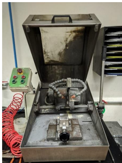
Fig. 3.6: Cutting machine used for material preparation
