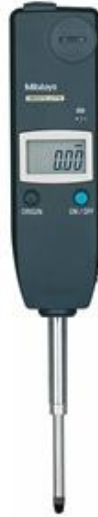
Fig. 4.17: The comparator used to verify the planarity of the samples before the wear test [21]
