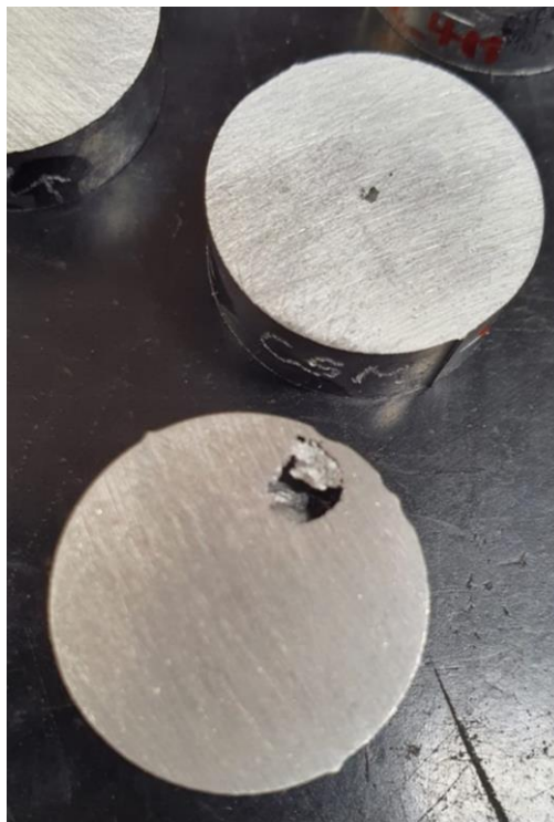
Fig. 4.21: Porosities formed in the High-Fe alloy
