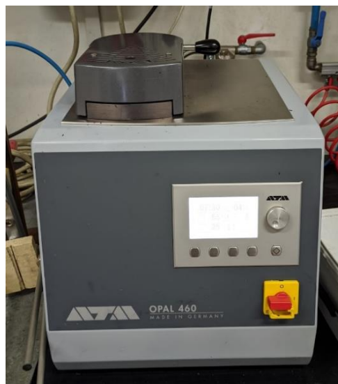
Fig. 3.8: Embedding machine used to incorporate the alloy into the resin
