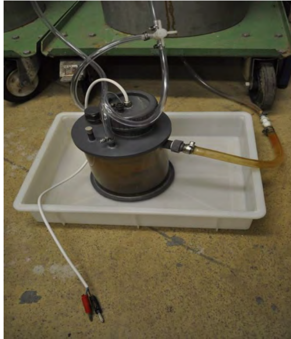
Figure 12 Leachate collection tank
