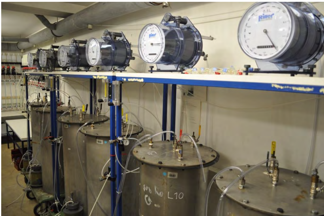
Figure 14 LSR installed inside 36°C conditioned room
