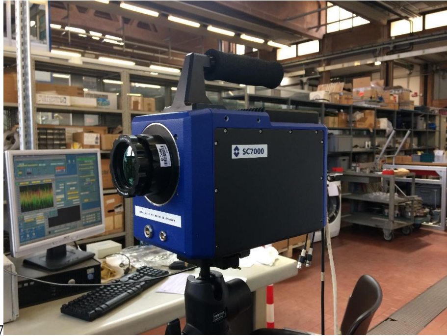
Figura 3.2. Termocamera FLRI SC7000
