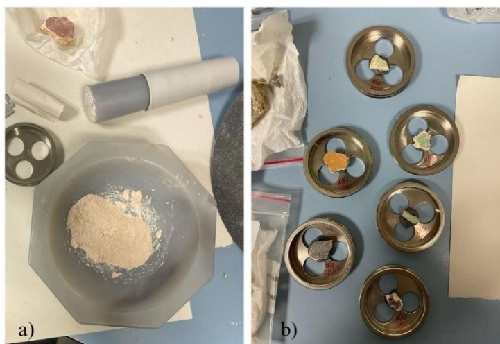
Figure 10. a) Powder of 0.8g of sample, grinded using pestle and mortar, b) Sample fragments placed on metal disc, ready to be set in the diffractometer. Department of Geosciences, Padova.
