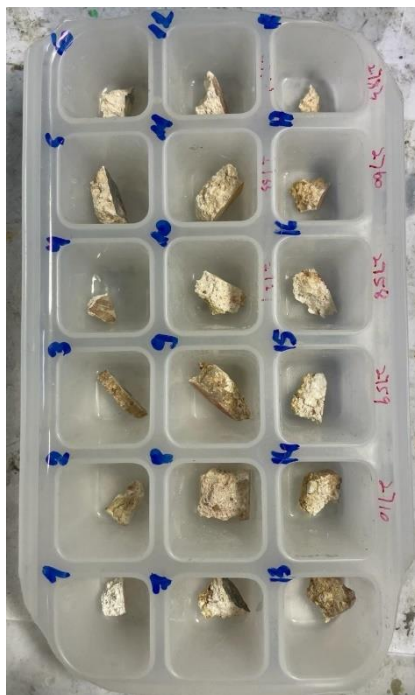
Figure 7. Samples of fragments placed in molds, before the pouring of resin, Department of Geosciences, Padova, Italy.
