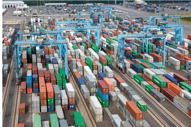
Figure 31: block stacking Source: konecranes.com
