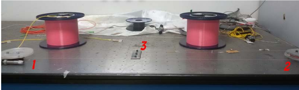
Figure 4.5: Picture of the strain measurement setup: it is possible to notice two fiber coils, the plastic wheels (1 the movable, 2 the fixed) and the fiber positioned in between. 3 is the metal plate.
