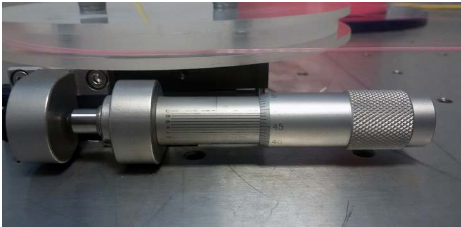
Figure 4.6: Picture of the reel put under the plastic wheel in order to move it and strain the fiber leant on it.
