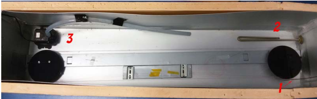
Figure 4.10: Complete setup for both temperature and strain measurements: in the middle there is the strain-specific setup, 1) is the thermocouple, 2) the electrical resistance and 3) the air pump.
