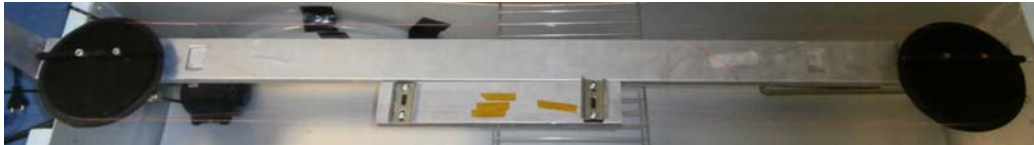
Figure 4.7: Strain modifier: at the ends of the aluminum bar there are the two black plastic wheels (to the left the movable, to the right the fixed) with fiber around them, in between two metal plates to fix the FUT.
