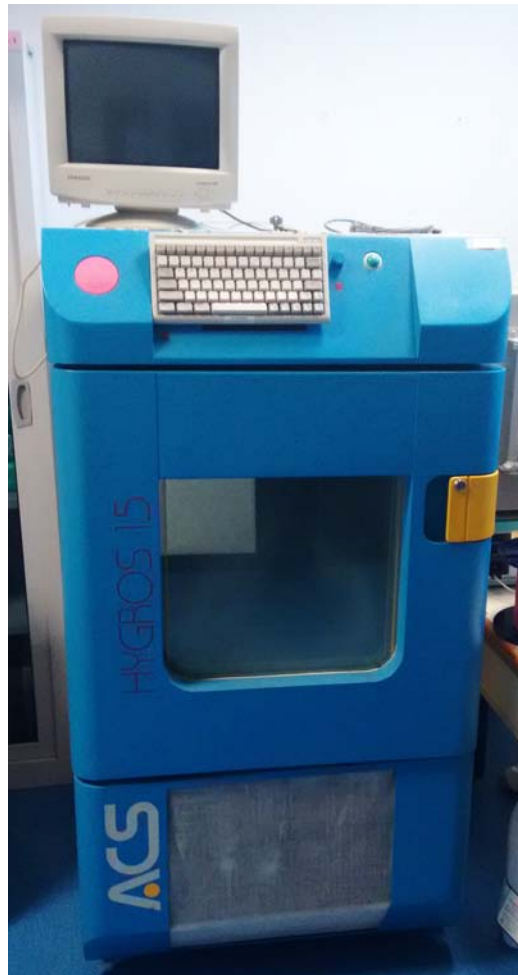
Figure 4.4: Picture of the climatic chamber used for temperature only measurements.
