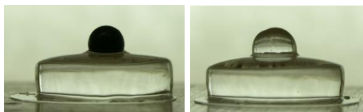
Figure 6.3. PAA 2 indented with plastic sphere (left) and glass sphere (right).
