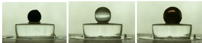
Figure 6.4. PAA 6 indented with plastic (left), glass (centre) and steel sphere (right).
