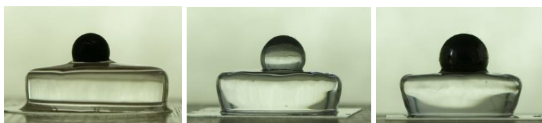
Figure 7.5. PAA-OH 1 indented with plastic sphere (left), PAA-OH 2 indented with glass sphere (centre) and PAA-OH 3 indented with steel sphere (right).
