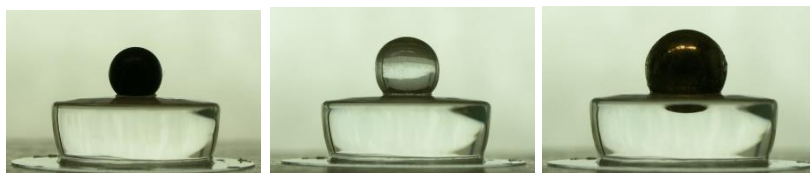
Figure 6.3. PAA 3 indented with plastic (left), glass (centre) and steel sphere (right).
