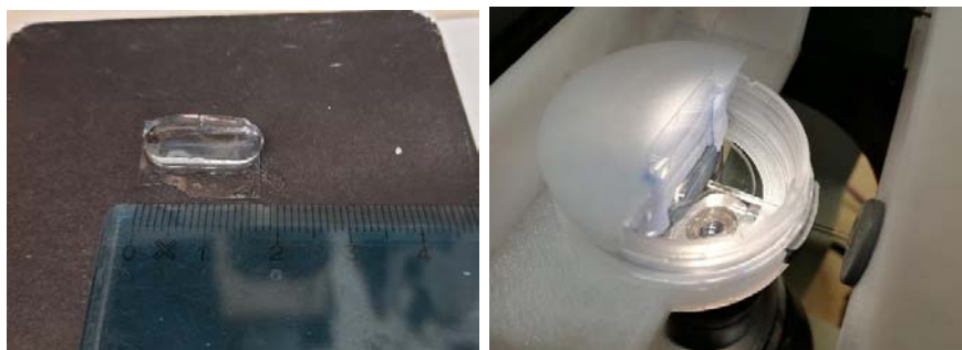
Figure 5.2. Sample of PEG hydrogel (left) and set-up (right) for the micropipette aspiration.
