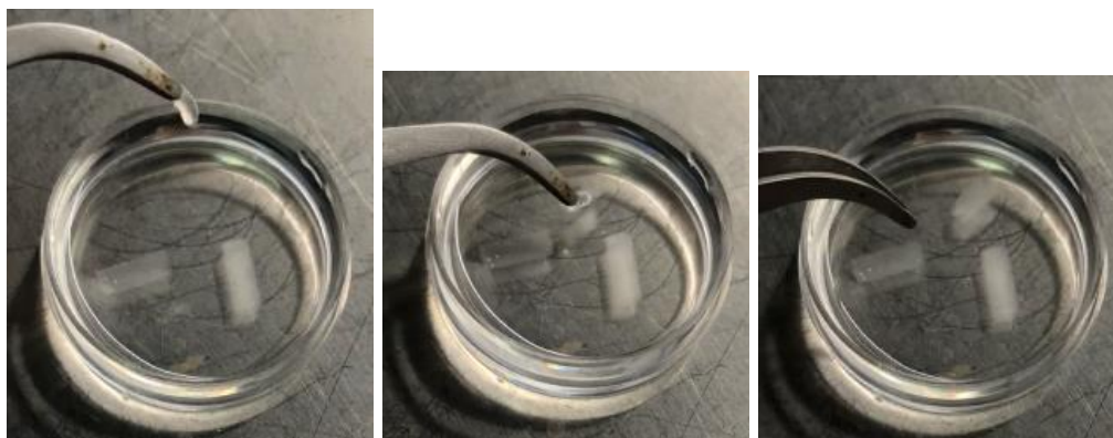
Figure 7.18. Swelling of cryogels.
