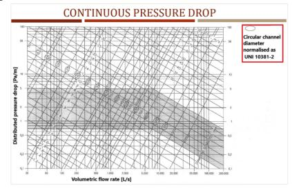
*Figure 4.14 – pressure drop as a function of the flow rate and diameter*
