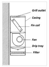
Figure 4.9 – general scheme of fan coil
