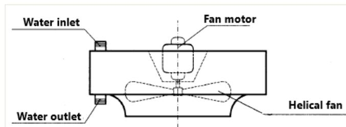
Figure 4.8 – vertical projection type [20]
