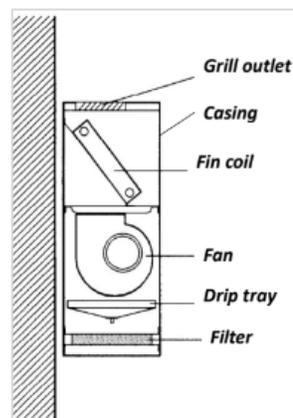
Figure 4.9 – general scheme of fan coil
