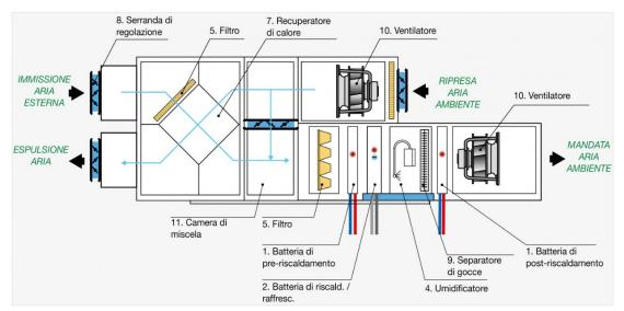
Figure 4.15 – typical scheme of AHU [25]
