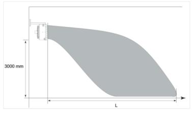
*Figure 4.10 – air penetration of air heaters* [21]
