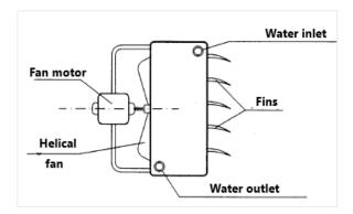
*Figure 4.7 – horizontal projection type* [20]
