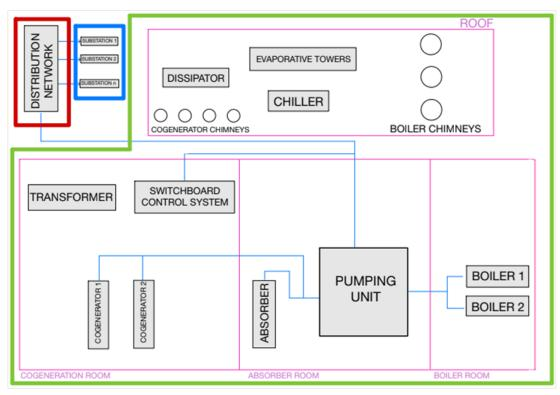
Figure 2.4 – Block scheme of the district heating plant of Padova
