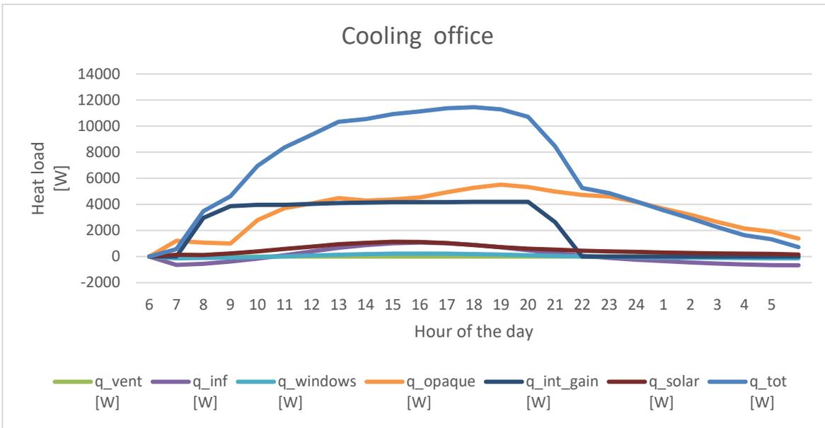
Figure C.1 – cooling profile of the office
