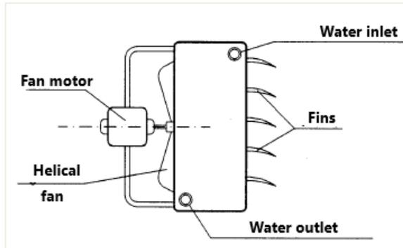
Figure 4.7 – horizontal projection type [20]
