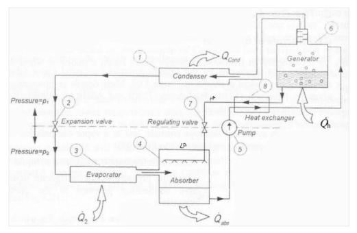
Figure 2.7 – General scheme of an absorption chiller [7]
