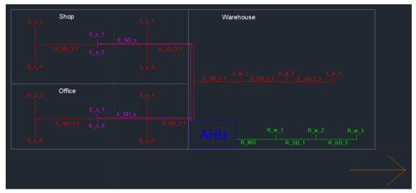
*Figure 4.13 – sketch of the air distribution system*
