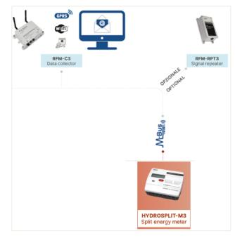
Figure 3.3 – scheme of the infrastructure from the meter to the concentrator [15]
