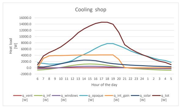
The peak power for the cooling is determined as the maximum value calculated over the course of the entire day for each room. With regard to the shop, the maximum value is recorded at 5 p.m.
