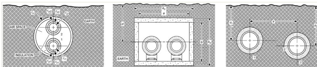
*Figure 2.2 – Possible configuration of the distribution line*
