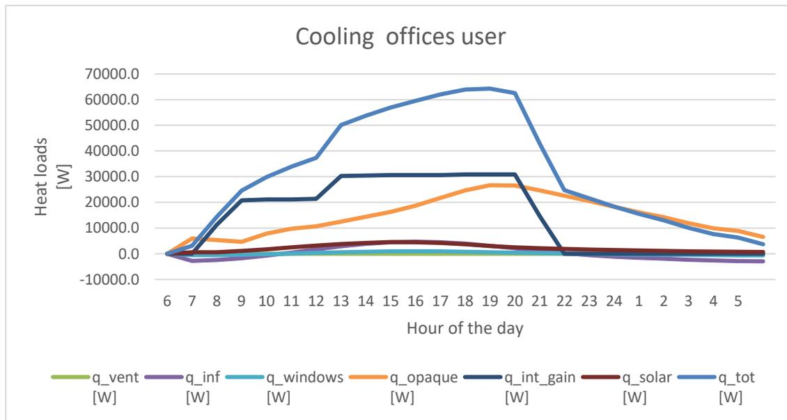
Figure 4.5 – cooling profile of offices user
