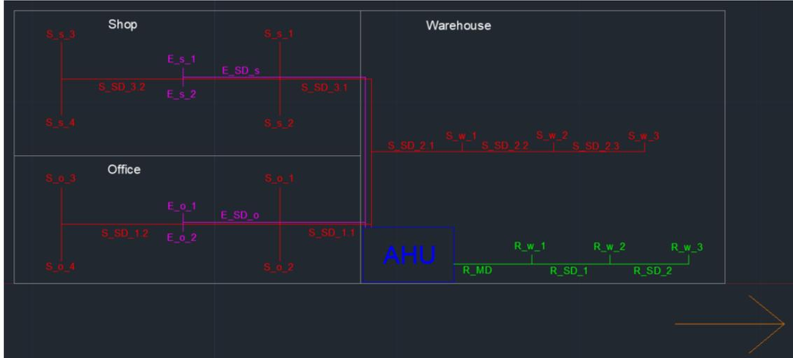
Figure 4.13 – sketch of the air distribution system
