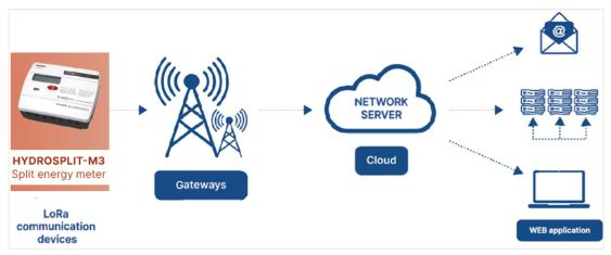
Figure 3.1 – example of LoRaWan system
