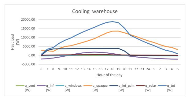
*Figure C.2 – cooling profile of the warehouse*
