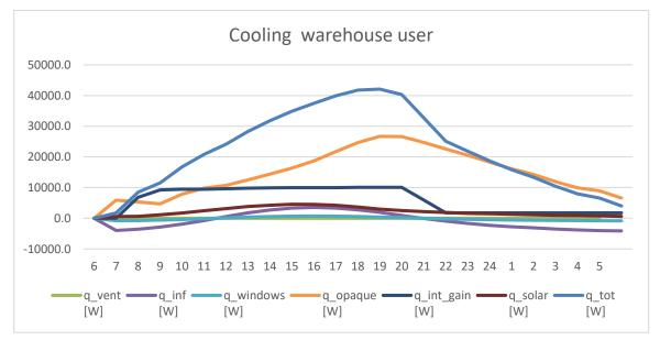
*Figure 4.6 – cooling profile for warehouse user*
