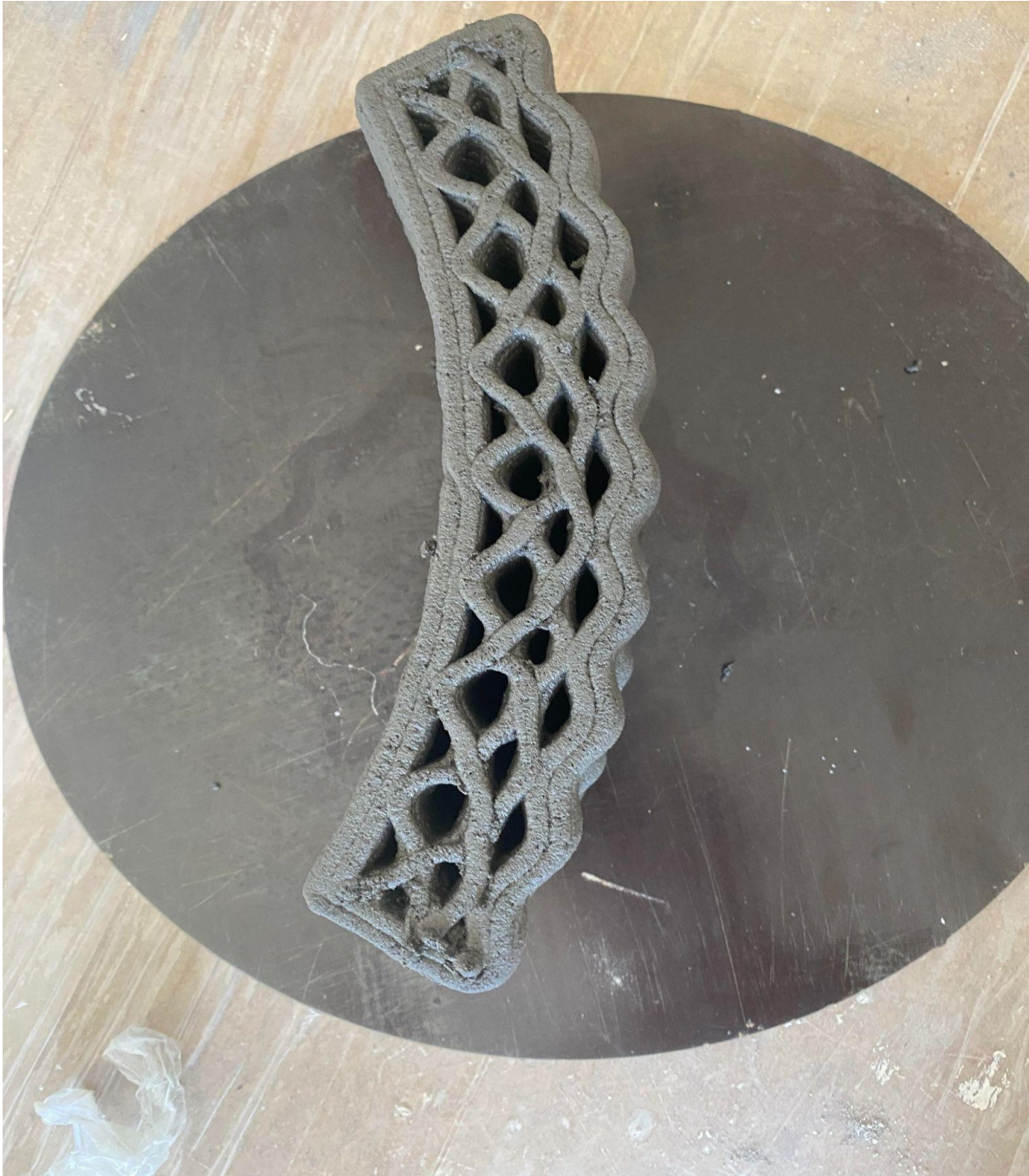
Figure 4.4b: Top view of scaled up print using Lunar Regolith based geopolymer
