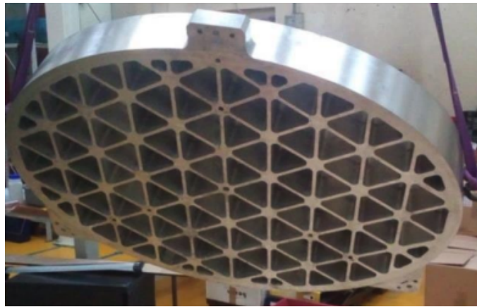
Figure 3.2: Honeycomb structure of M1 for mass reduction. Source: ESA.
