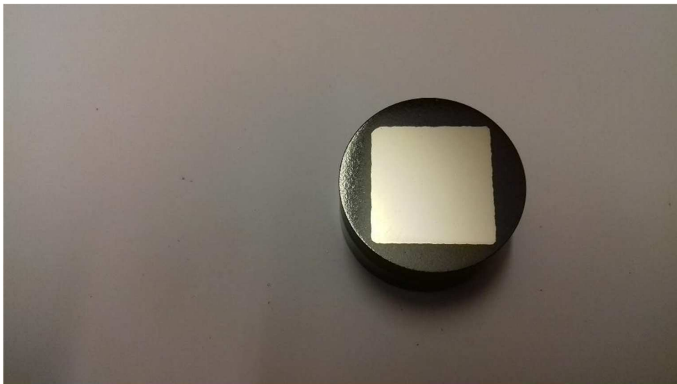
Figure 2.4: Sample mounted in a conductive resin
