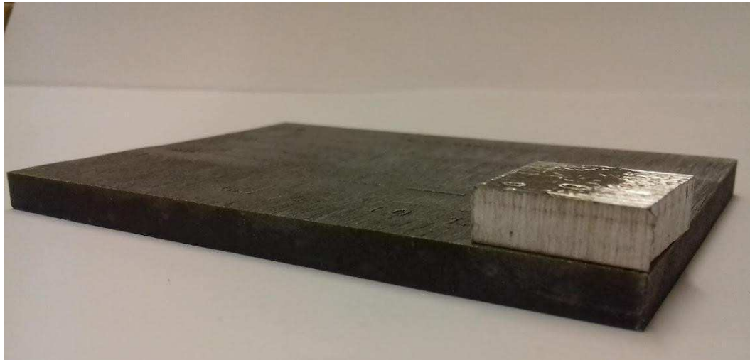
Figure 2.1: Sample arrived from Pretoria (100x40 mm) on the bottom. Sample cut in Jönköping University (20x20 mm) on top
