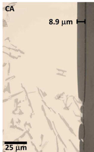
Figure 4.7: AlSi10Mg made by casting cross section, after 20 min of anodizing[35]
