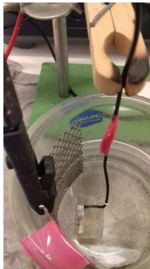
Figure 2.5: Sample during the anodizing process
