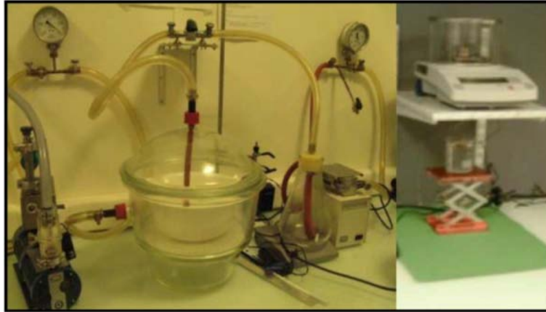
Figure 2.14: Porosity measuring device: a) the bell hermetic glass, left; b) the electronic balance to the right.
