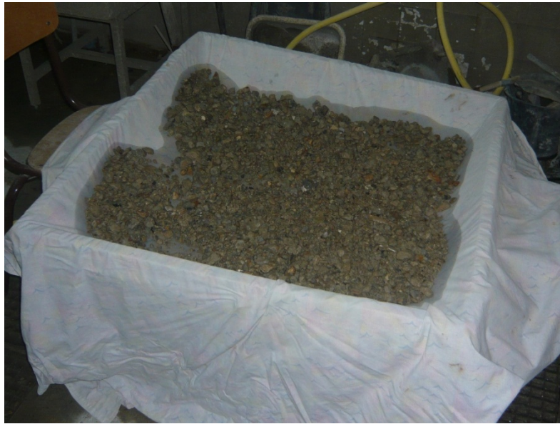
Figure 2.3: Recycled aggregates in a strainer.
