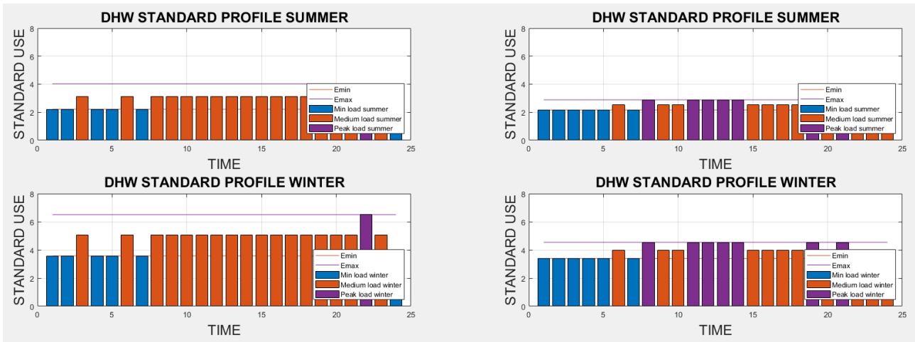
Figure 81 Standard profiles in winter and in summer for days of group 1 (left) and group 2(right) in building 10686, Tartu.
