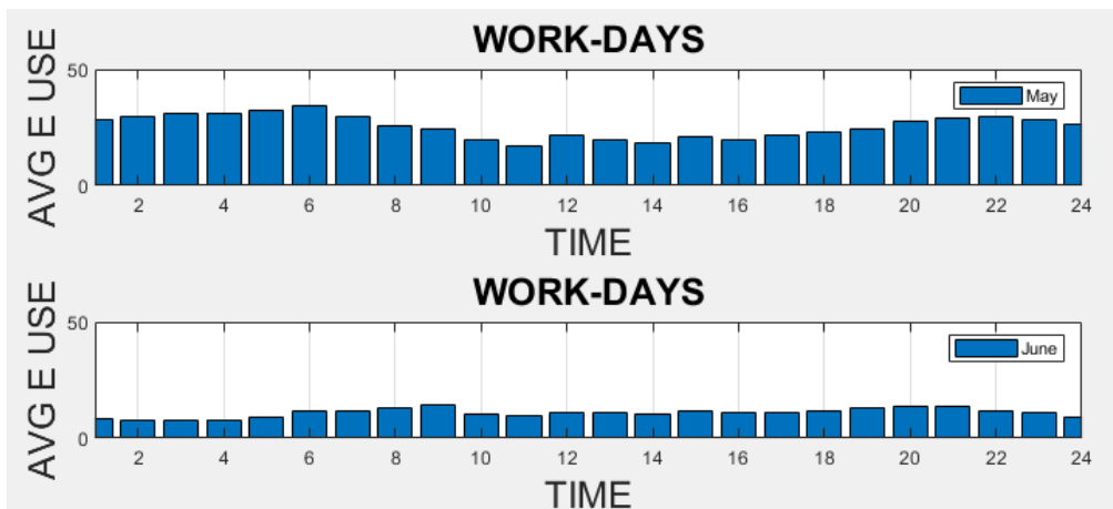
Figure 17 An example of DHW mean plot analysis of workdays of May and June
