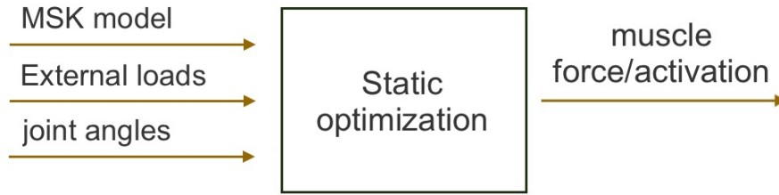
Figure 3.7: Static optimization block diagram
