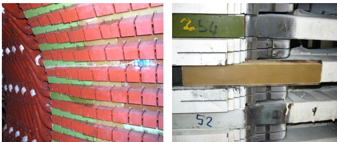
Figure.6.1: Step-frame of the stator core at the end of the stator winding (first 750 MVA, second 370 MVA, 2 poles generators) 72 .
