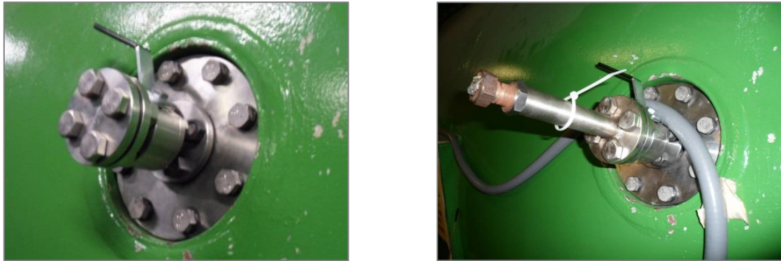
Figure.3.7: The insertion valve and the rail of the probe.
