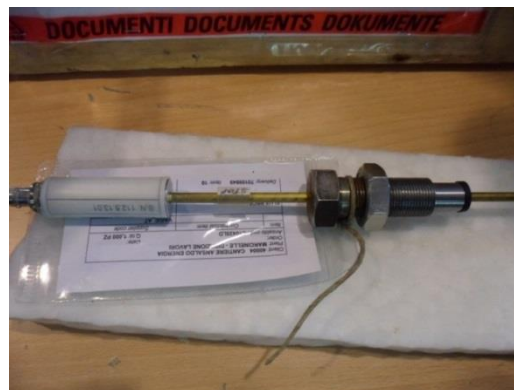
Figure.3.3: External part of the flux probe.
