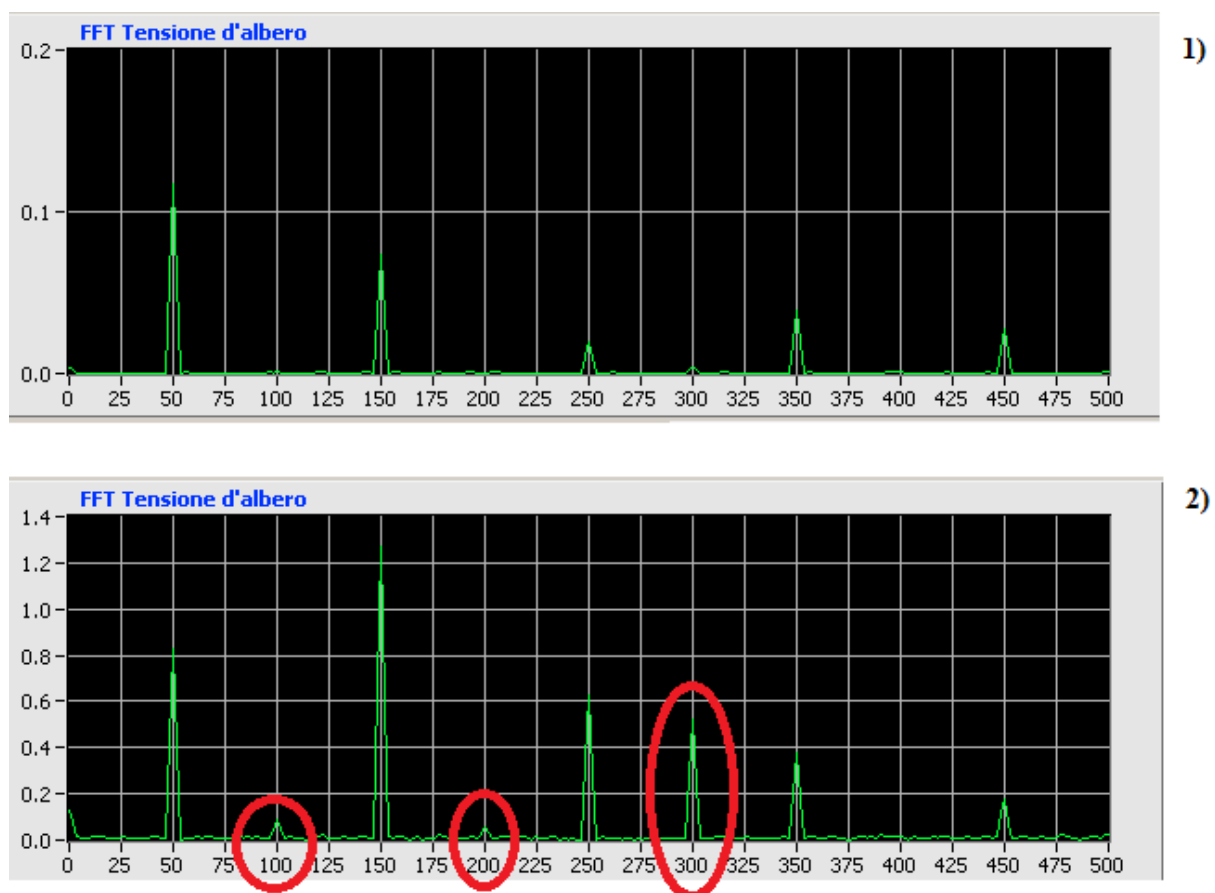
Figure.4.13: Shaft voltage frequency spectrum: 1) good operation, 2) fault operation (presence of even harmonics).
