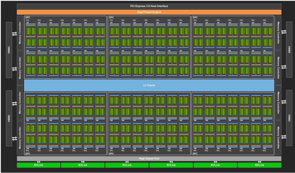
Figure 7: Complete Volta GV100 GPU architecture
