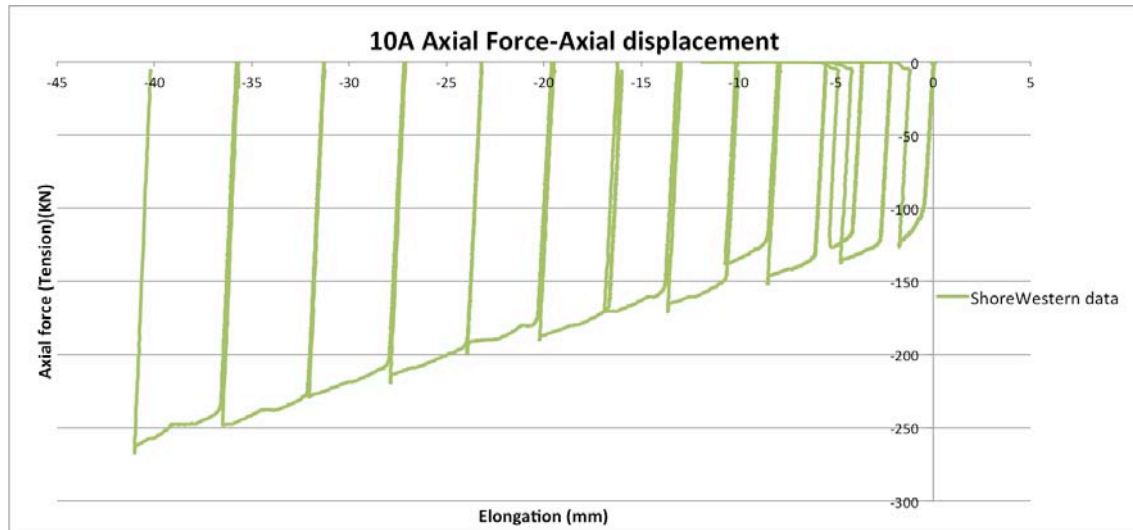
Figure 12.10: specimen 10A, Lode angle \theta=40^\circ , axial force-axial displacement
