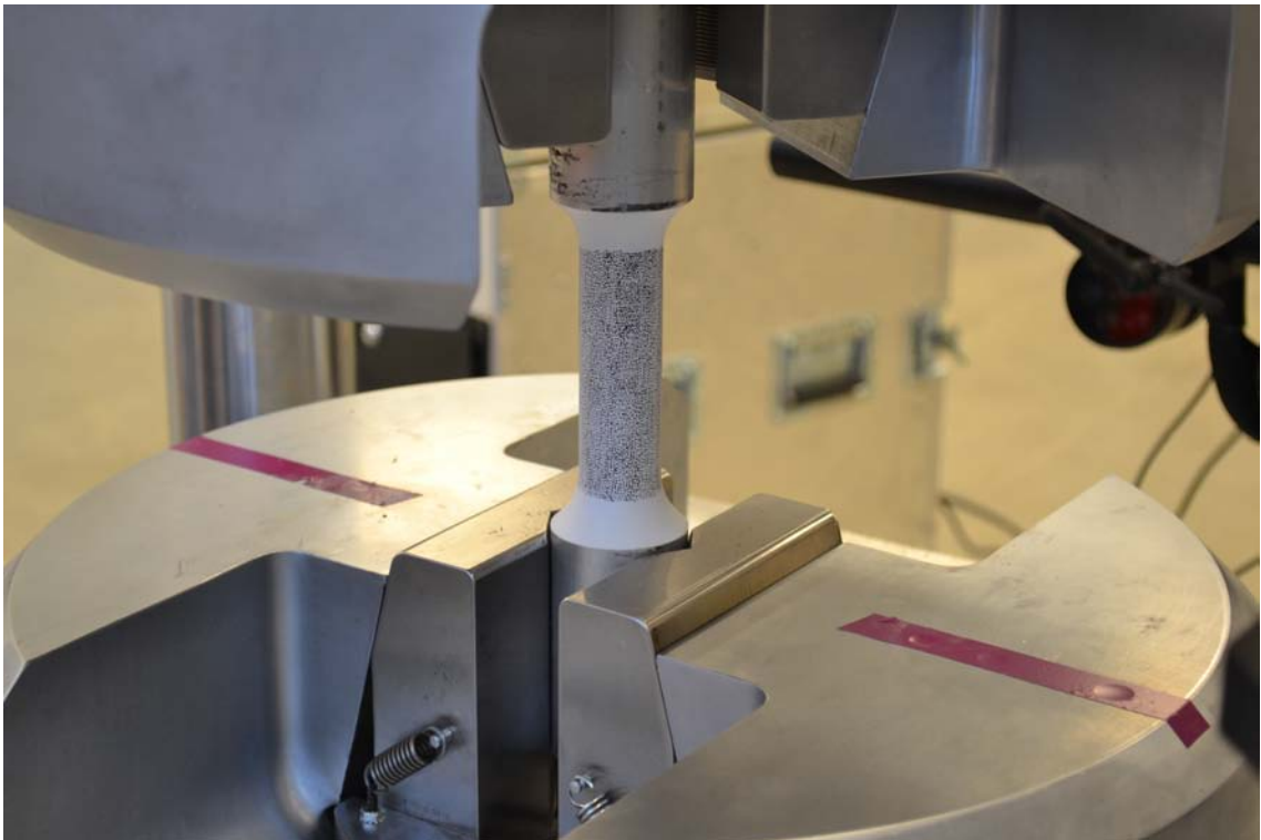
Figure 11.54: specimen 4A in the grips
