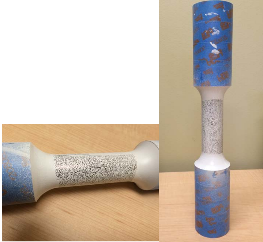
Figure 10.5: specimens painted with a white varnish and black random dots
