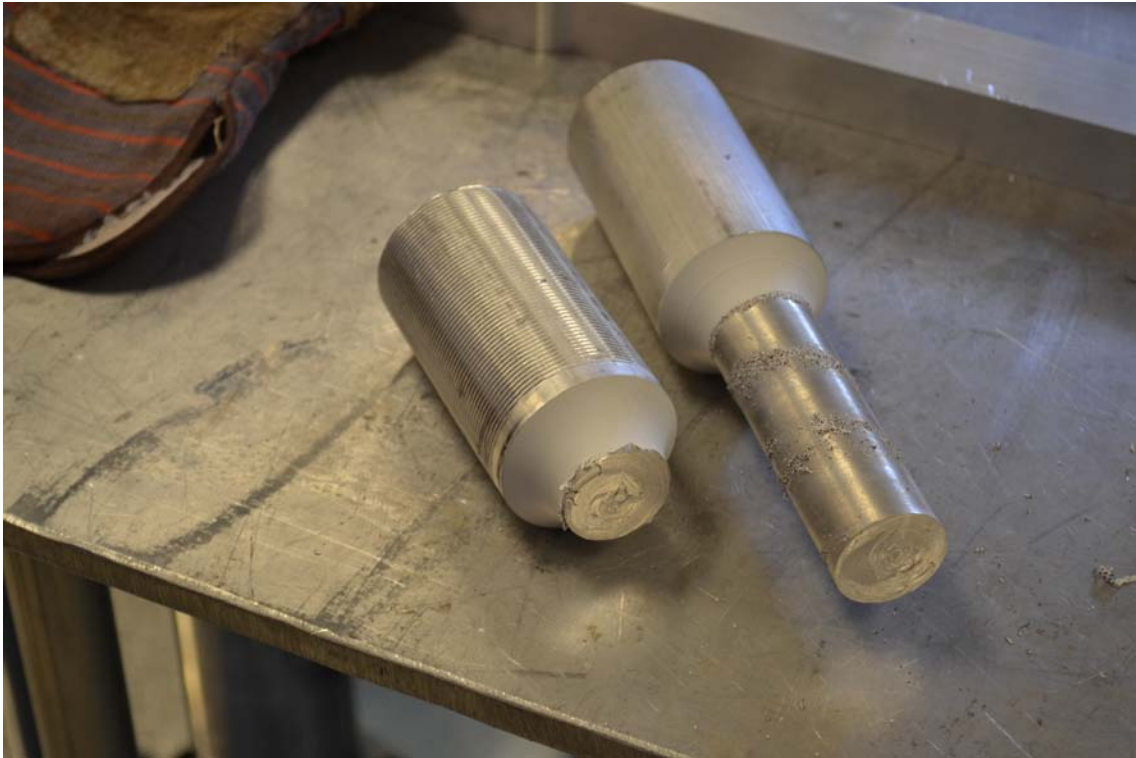
Figure 11.56: collapse of the specimen
