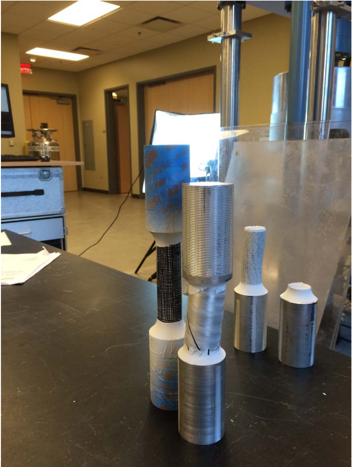
Figure 11.71: specimen after 14 cycles; a shortening of 3.8 cm is noticed.
