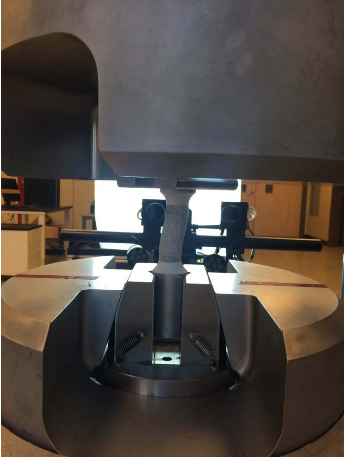
Figure 11.88: specimen 8A under compression-torsion
