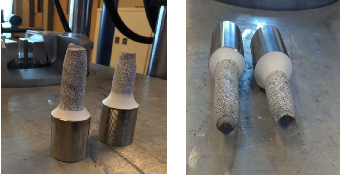
Figure 11.13: failure of the traction specimen
