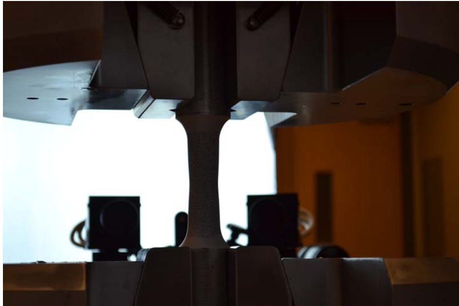
Figure 11.10: tension test, starting of the necking
