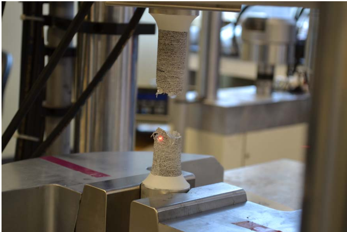
Figure 11.45: collapse of the specimen
