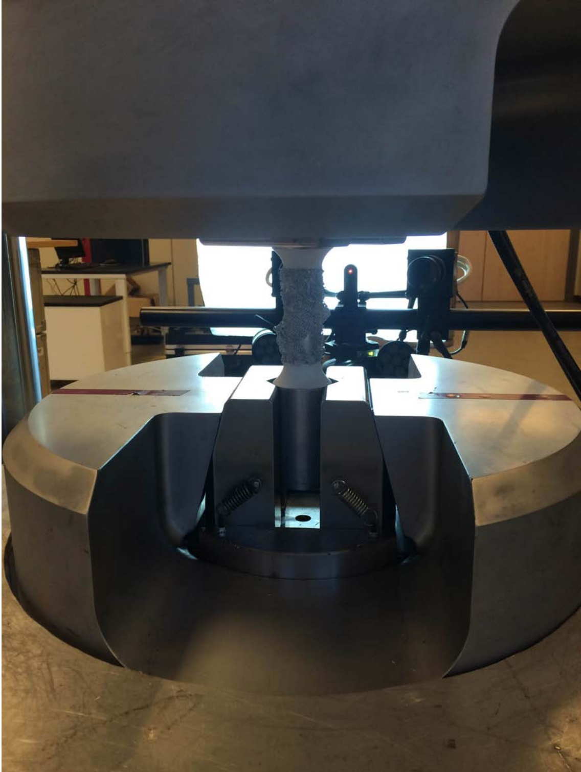
Figure 11.68: specimen 10A in the grips after 3 cycles
