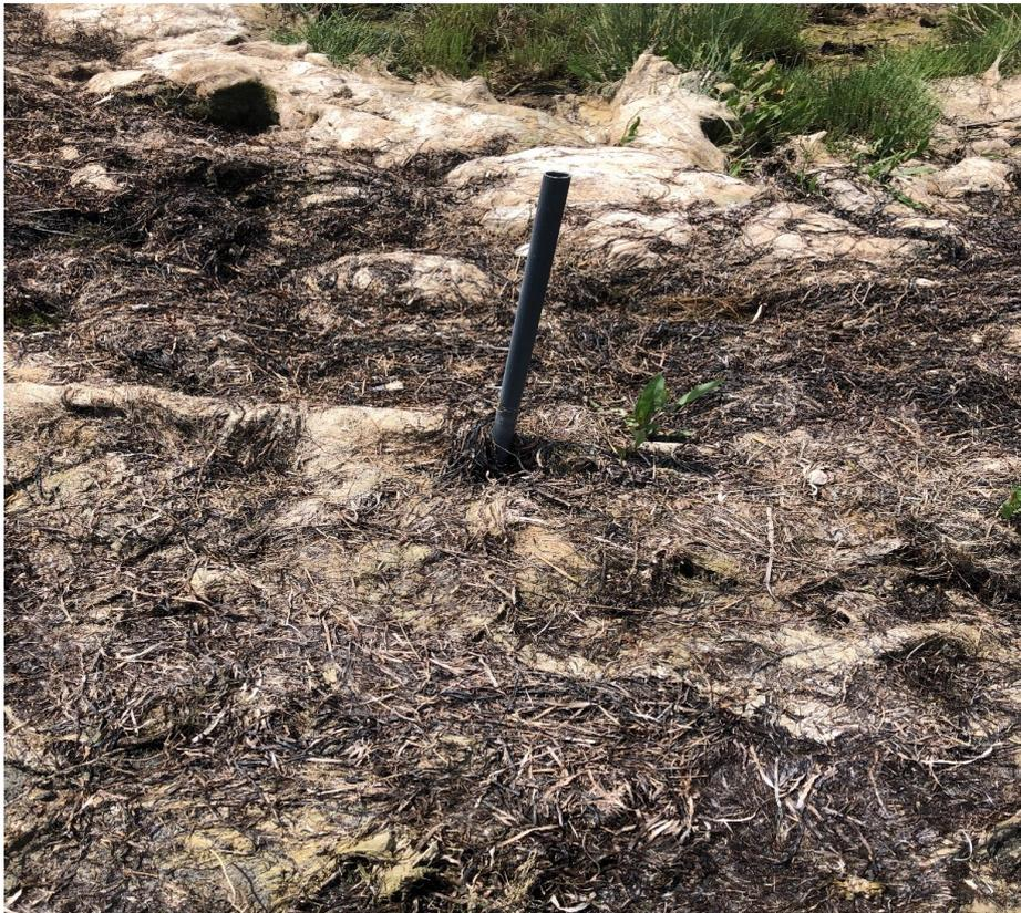
Figure 3. Wrack treatment with the temperature ElectricBlue EnvLogger V2.4 inside and the stick to fix it on site 3 in Cà Manzo.
