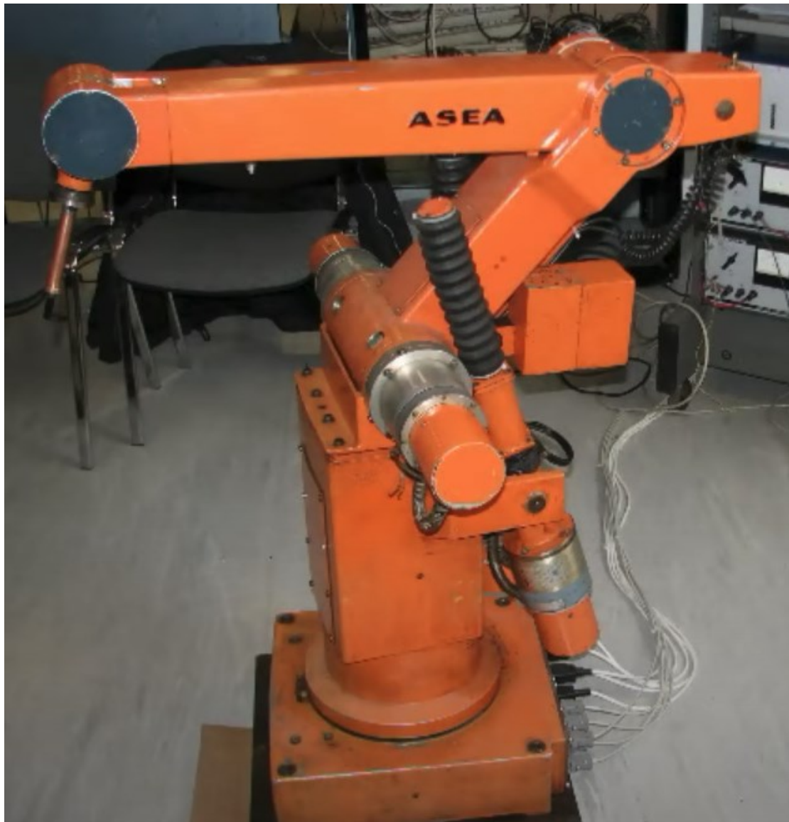
Figure (2.4) IRB-6 developed by ASEA (ABB now).
