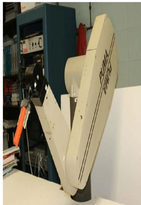
Figure (2.3) shows the PUMA Robot.
