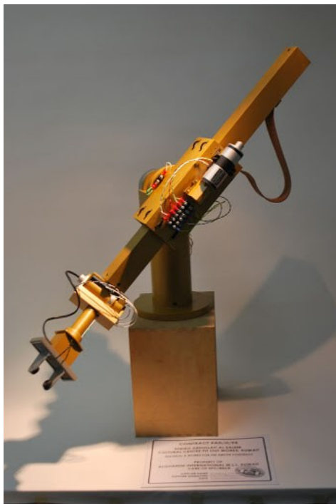
Figure (2.2) the Stanford arm.
