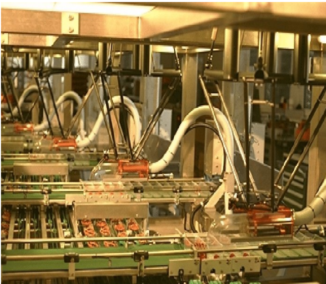
Figure (2.7) Six Delta in Swiss Company Demaurex's Production Line.
