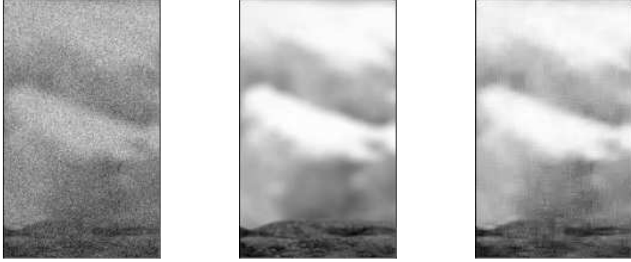
Figure 2.6: image noised, original and denoised, MSE < 0.004
