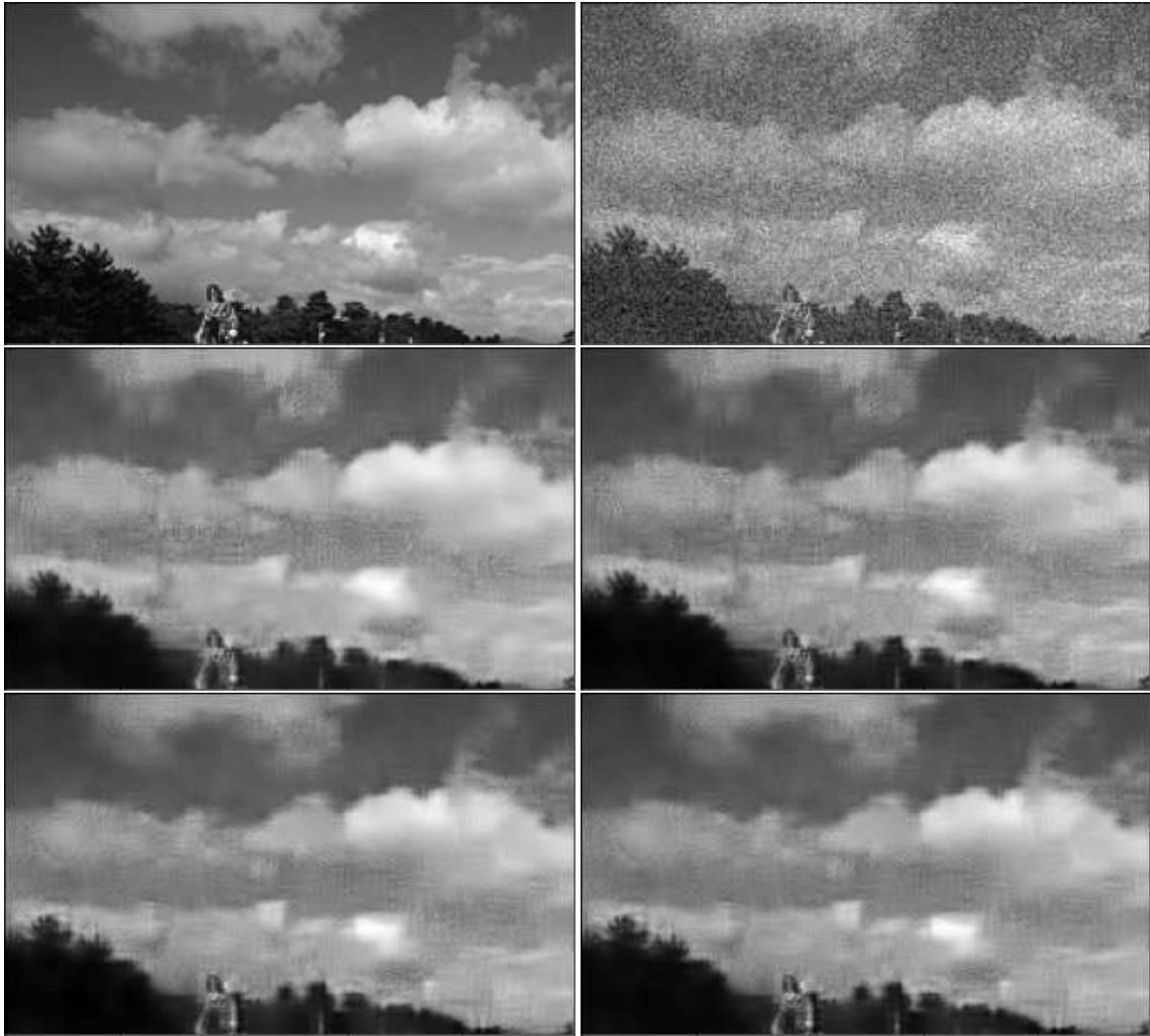
Figure 3.8: Comparison of implemented denoisers applied to the input image: (a) Top left: Original clean image, (b) Top right: Image with added noise, (c) Bottom left: Image denoised using D_{MSE} , (d) Bottom right: Image denoised using D_{MIX}^{0.7} , (e) Bottom right: Image denoised using D_{MIX}^{0.6} , (f) Bottom right: Image denoised using D_{MIX}^{0.69} . In this figure we added also the outputs for D_{MIX}^{0.6} and D_{MIX}^{0.69} , to visually show that, although the highest values of SSIM and PSNR of these compared to D_{MIX}^{0.7} , image (d) results less smooth and presents some splotchy artifacts. However, it preserves better structures, for examples, the different shades in the clouds.
