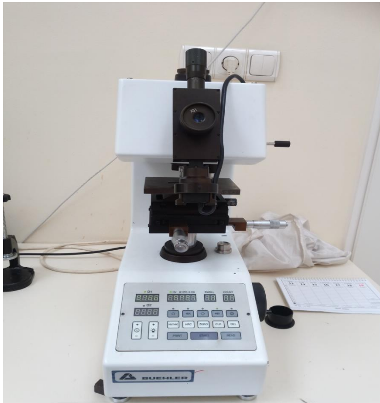
Figure 9. Micro hardness machine with electron microscope (Buehler company)
