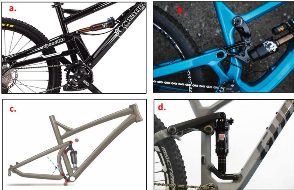
Figure 4. Different configurations: a) Single pivot, b) single pivot articulated c) virtual pivot d) Horst Link. Source: bikingpoint.es and others
