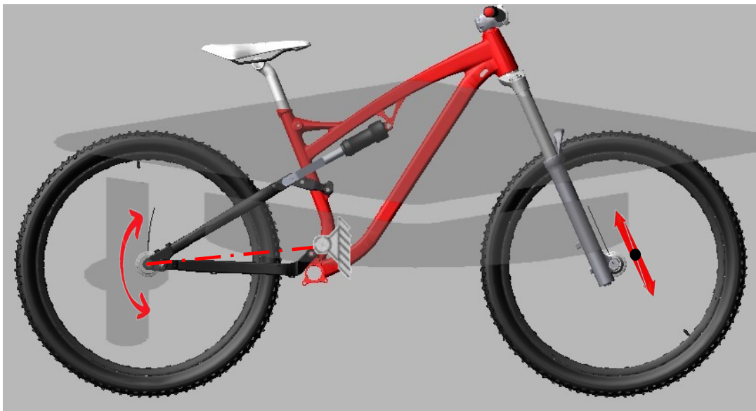
Figure 34. Trajectories of both front and rear suspensions. Source: own
