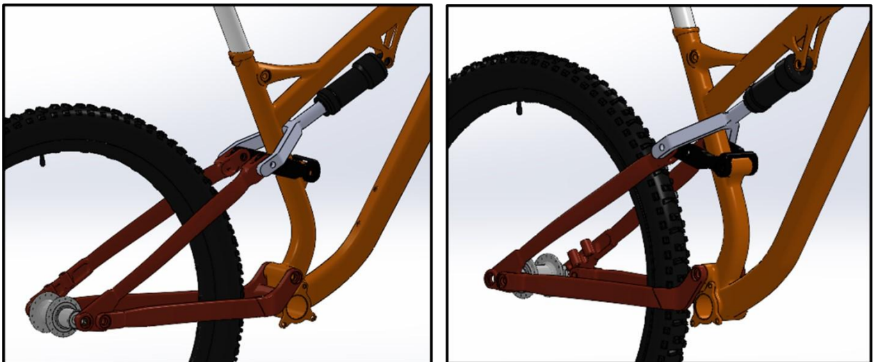
Figure 17. Rear suspension configuration of the simulation model.
