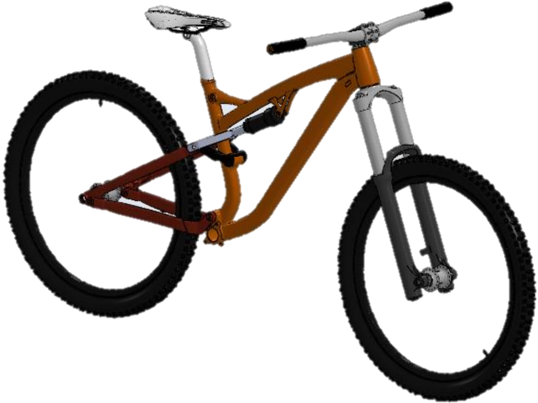
Figure 14. 3D model of the Specialized EPIC Pro used in the project.
