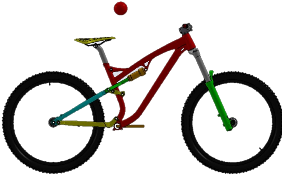
Figure 23. Body and bike modeling in Adams. Source: own
