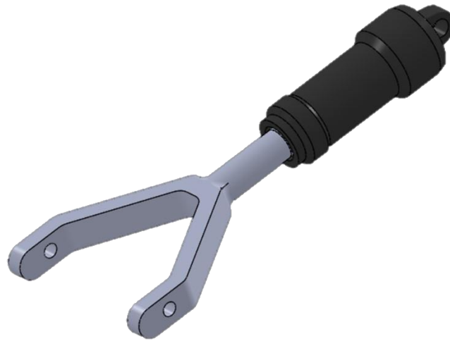
Figure 18. Own creation geometries of the rear suspension. Source: own
