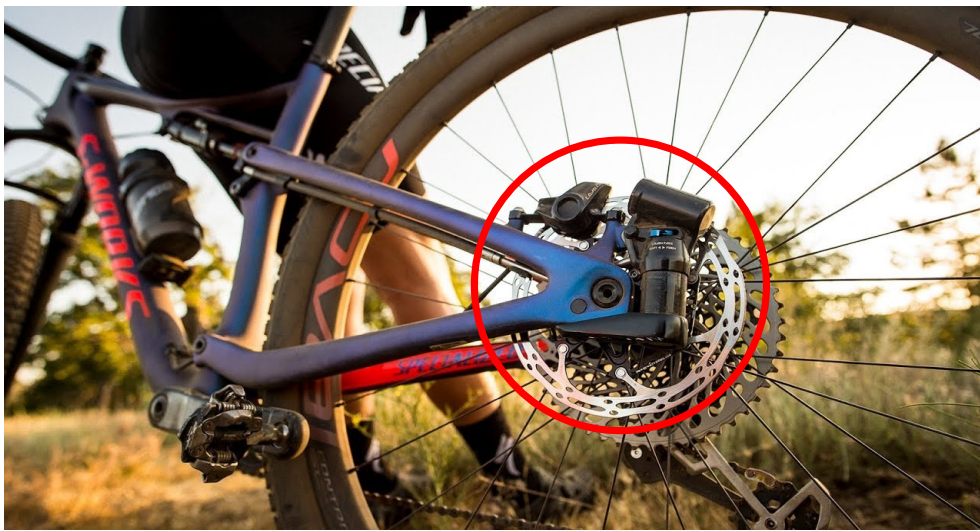
Figure 8. Old version of the Brain, located in the rear wheel hub. Source: Specialized
