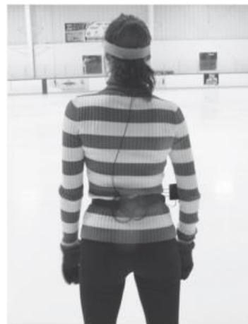
*Fig.36 "Accelerometer placement"*
