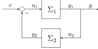
$$\Sigma_{ret} = \begin{cases} \dot{x}_1 = f_1(x_1, -g_2(x_2, g_1(x_1)) + r) \\ \dot{x}_2 = f_2(x_2, g_1(x_1)) \\ y = g_1(x_1) \end{cases}$$
