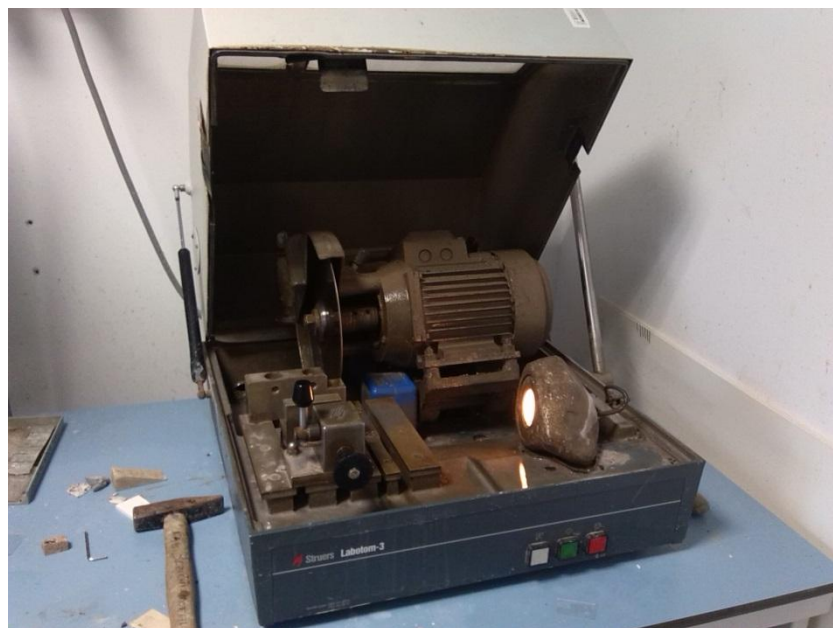
Figure 4.2: the Struers Unitrom-3 saw for small cuttings.
