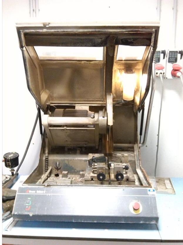
Figure 4.1: the Struers Unitrom-2 saw for big cuttings.
