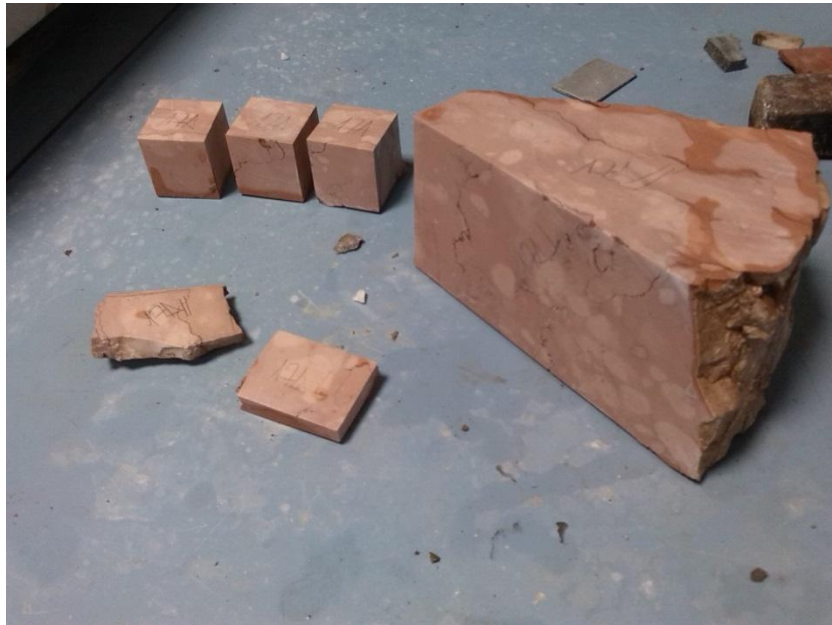
Figure 4.3: Cut samples for thermal property measurements, density and porosity measurements and thin sections.
