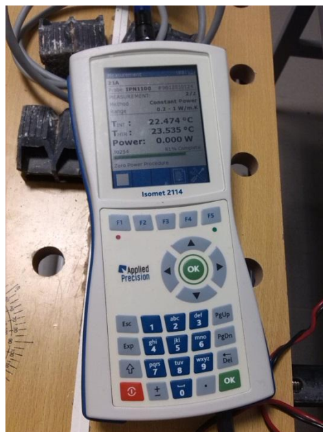
Figure 3.6: the ISOMET 2114 instrument for thermal conductivity measurements
