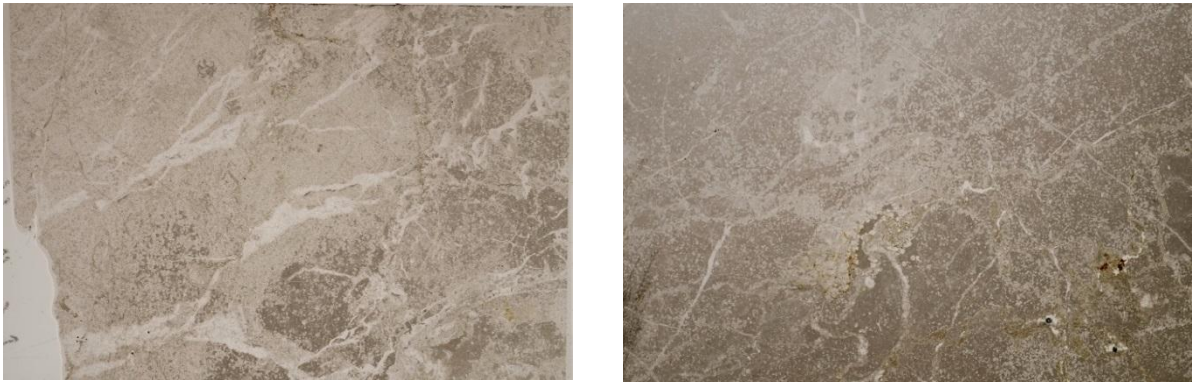
Figure 4.88: Thin sections of the sample 16A: a) section cut parallel to the stratification; b) section cut perpendicular to the stratification. Vertical side: 25 mm.
