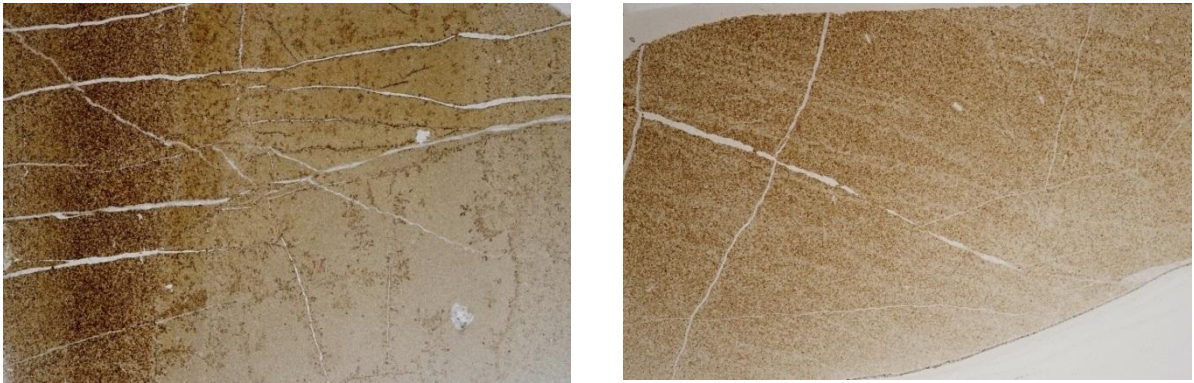
Figure 4.102: Thin sections of the sample 5A: a) section cut parallel to the stratification; b) section cut perpendicular to the stratification. Vertical side: 25 mm.
