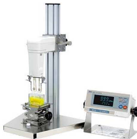
Figure 2.7 Vibro Viscometer SV-10 used in the test.
