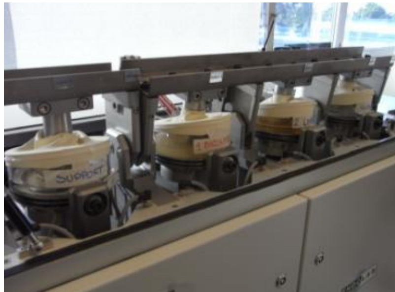
Figure 4.7 The knee joint simulator.
