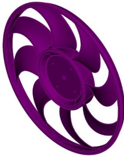
**Figura 2.20.** Modello CAD del cooling fan.
