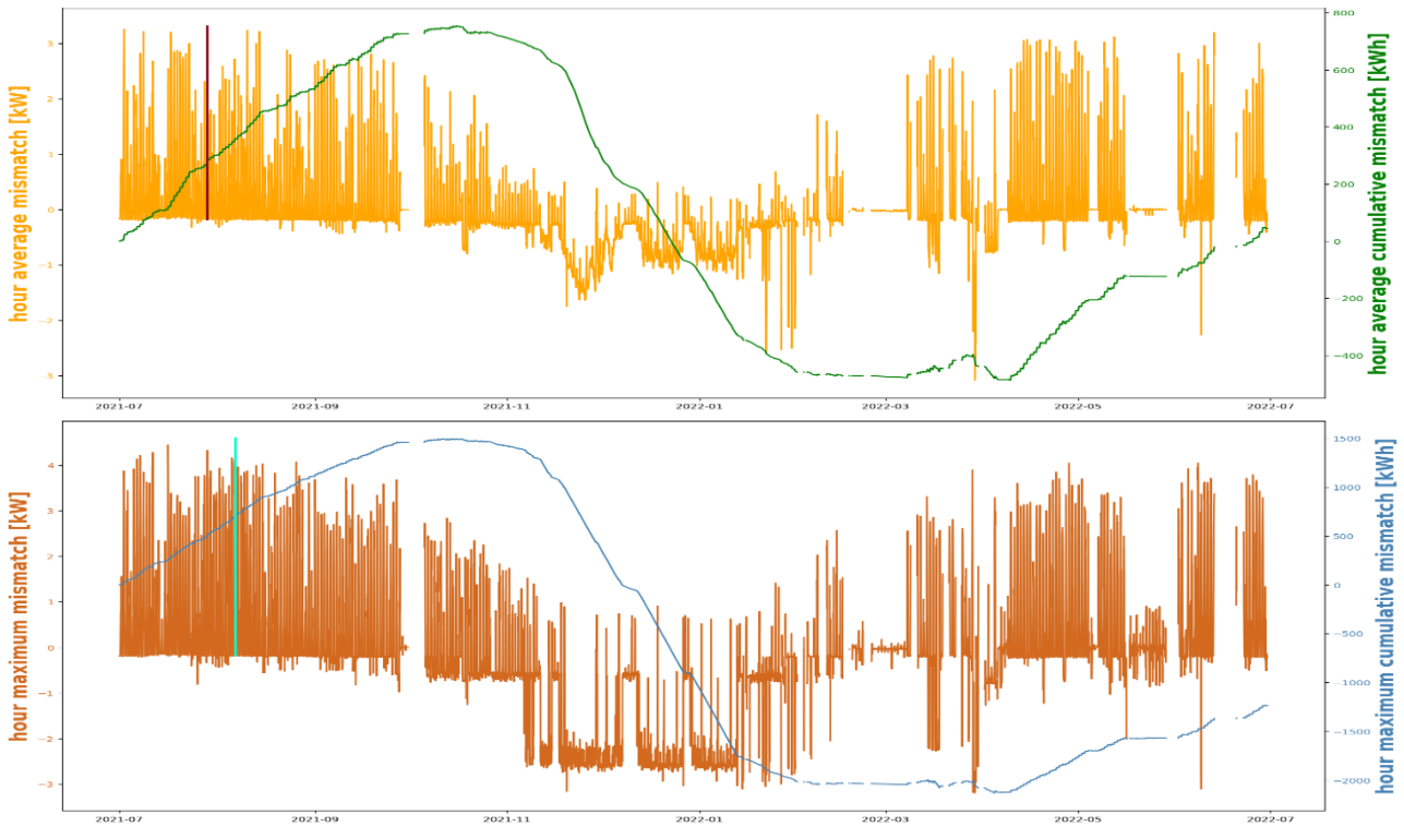
Figure 23: mismatch and cumulative mismatch in both case of average and maximum hour value
